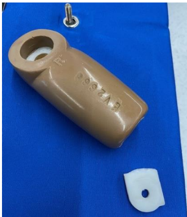
Figure 7: CRABI-12 Arm Joint Fracture at Elbow
