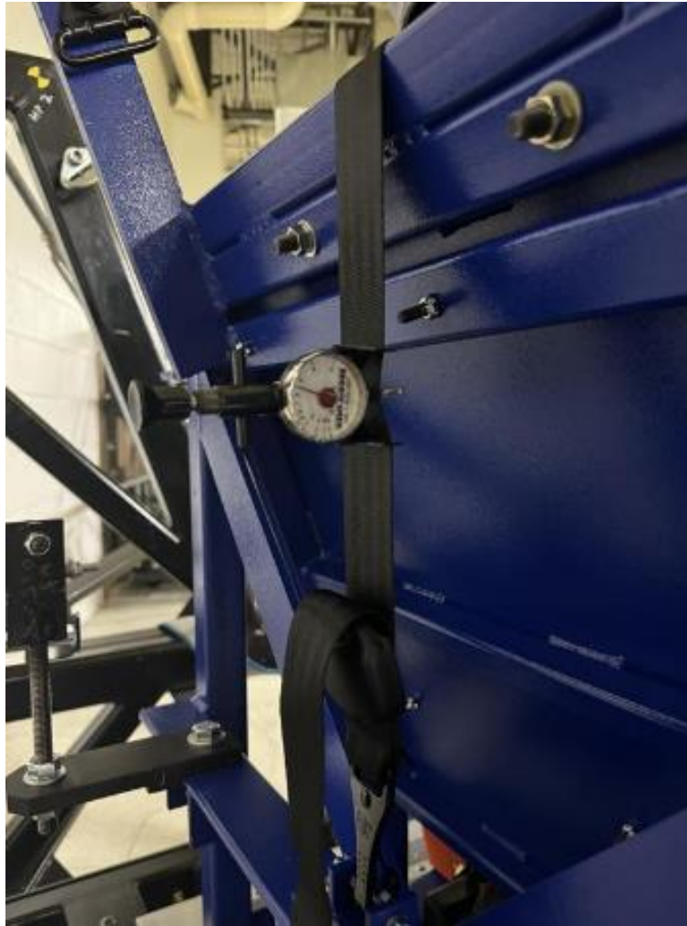
Figure 8. Tether Tension Measurement with 3-Prong Gauge at Proposed Location.
