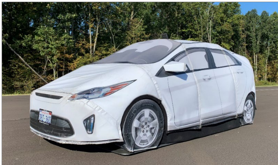
Figure 2. ABD GVT revision G vehicle test device secured to an ABD GST 120 robotic platform.
