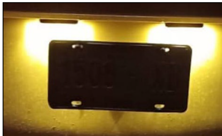
Figure 2: Overall view of the license plate when placed approximately 25 mm ahead of its normal position (test position), showing that it is not fully illuminated.
