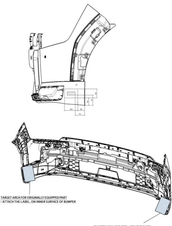
TARGET AREA FOR REPLACEMENT PART: ATTACH THE LABEL. ON INNER SURFACE OF BUMPER
