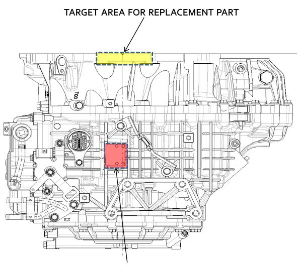
TARGET AREA FOR ORIGINALLY EQUIPPED PART
