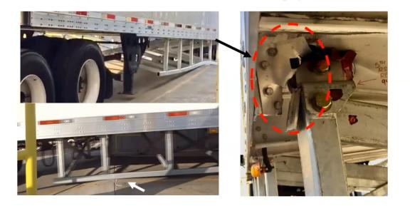
Angelwing Rigid Side Impact Guard Reduces Trailer Ground Clearance Resulting In High Centering Damage To Itself And The Trailer's Structural Integrity
