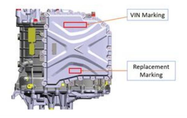
**NOTE:** Since the Electric Drive system (EDS) is one assembly which includes Motor, Transmission, and Inverter, it's like an engine that includes many parts (Block, cylinder heads, intake, etc); therefore, only one VIN label is affixed on EDS.
