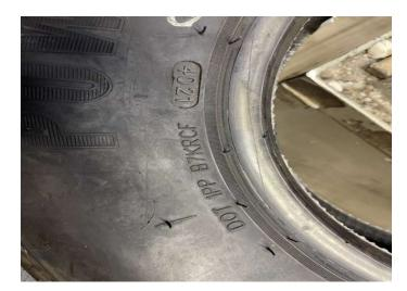
All of the other content within the TIN is accurate and complies with the TIN marking requirements. The tires otherwise conform to the performance requirements applicable to trailer tires. The date code discrepancy affects less than one week of tire production and the condition has been corrected in production. Hercules is not aware of any complaints, claims, or incidents related to the subject noncompliance.
