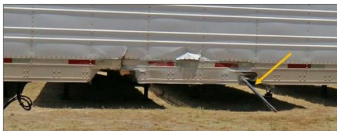
Figure 7. Closeup view of impact damage to the right side of the Utility semitrailer. The arrow indicates a segment of front windshield trim from the Tesla entrapped in the forward-most area of damage.
