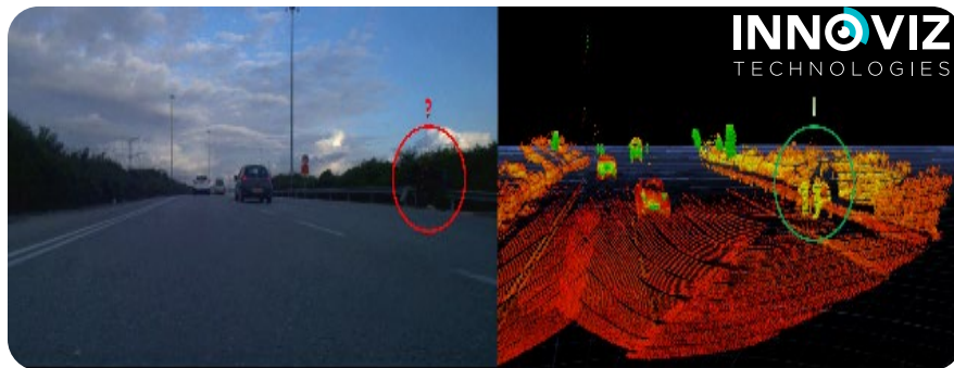
Figure 3 Camera vs. lidar detection in low light conditions
