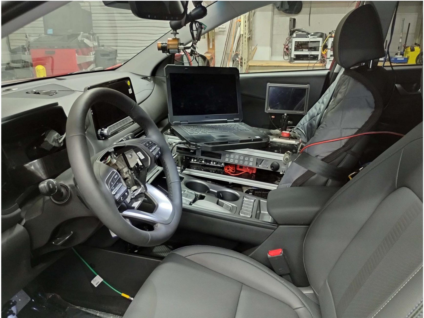
Figure A12. Computer Installed in Subject Vehicle
