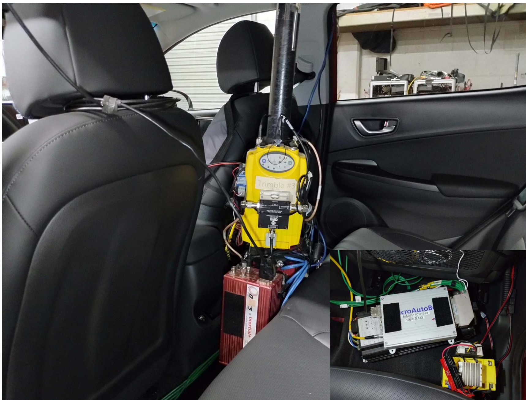
Figure A10. DGPS, Inertial Measurement Unit, and MicroAutoBox Installed in Subject Vehicle A-12
