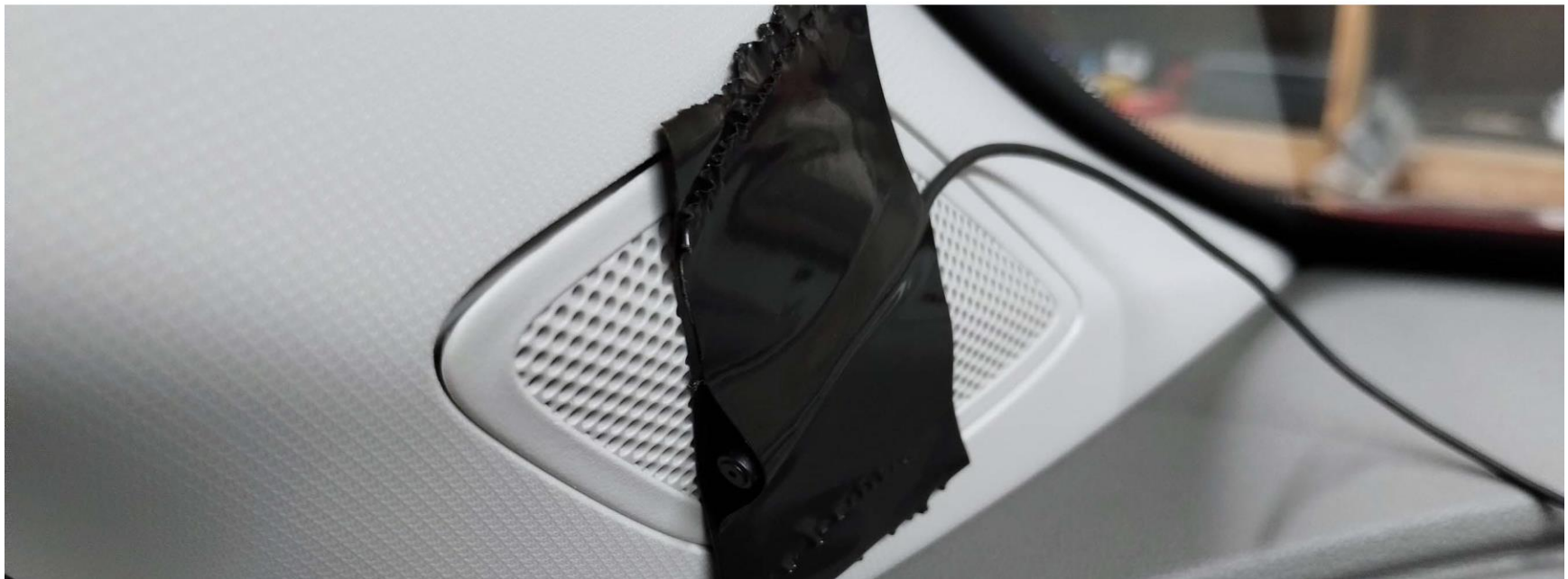
Figure A7. Sensors for Detecting Visual and Auditory Alerts
