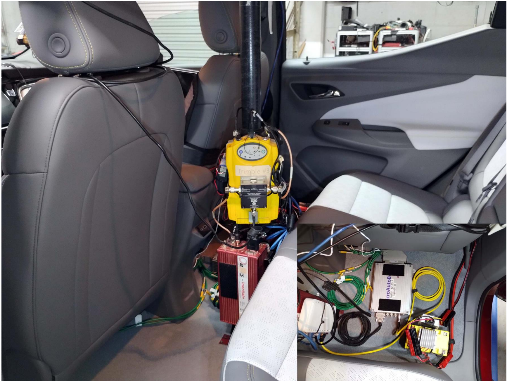
Figure A8. DGPS, Inertial Measurement Unit, and MicroAutoBox Installed in Subject Vehicle
