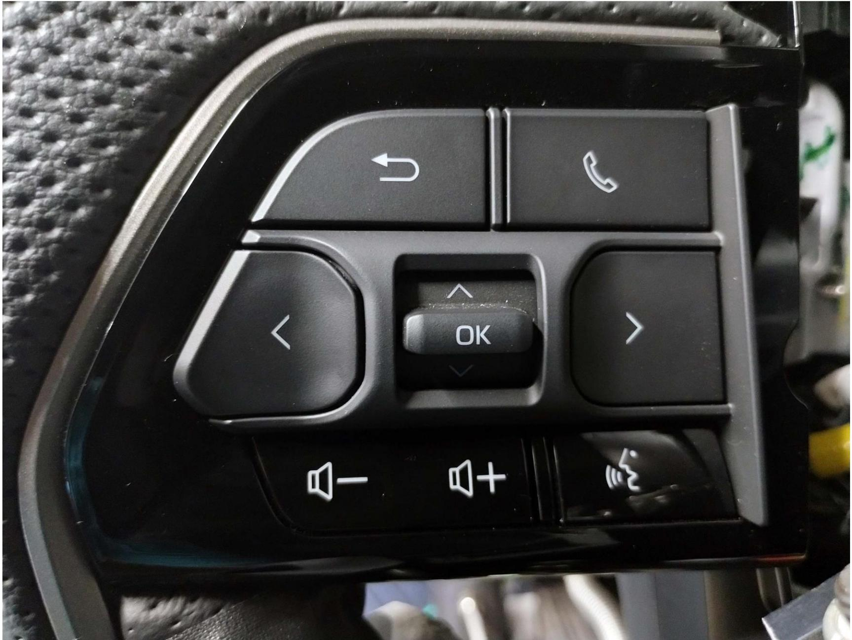
Figure A15. Steering Wheel Buttons
