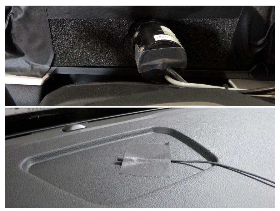
Figure A11. Sensors for Detecting Auditory and Visual Alerts A-13
