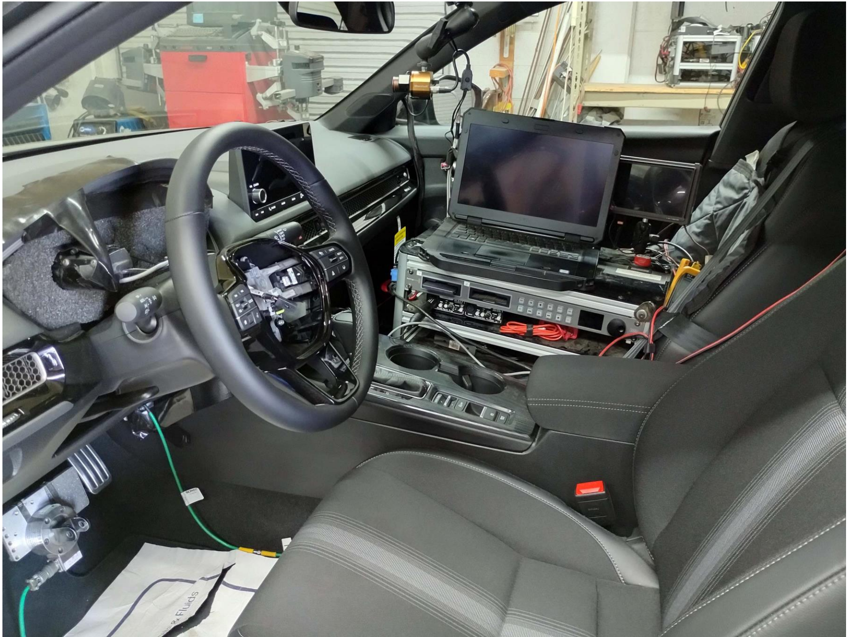
Figure A10. Computer Installed in Subject Vehicle
