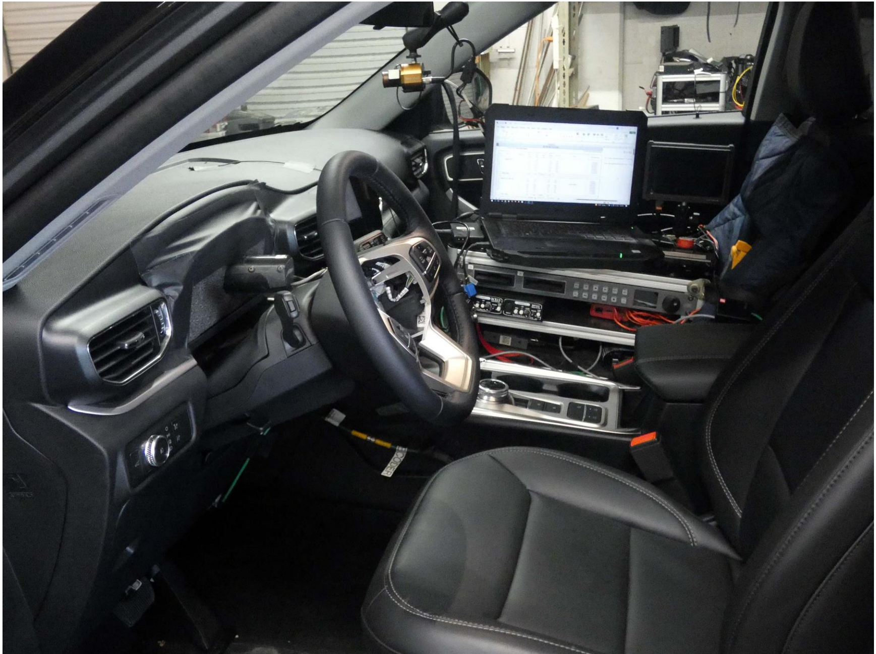
Figure A12. Computer Installed in Subject Vehicle
