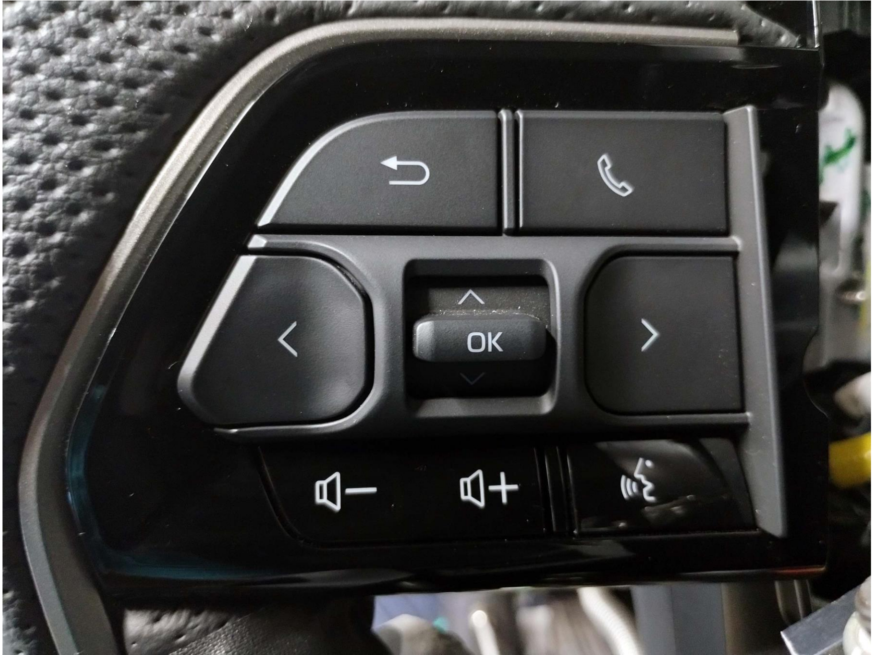
Figure A9. Steering Wheel Buttons for Adjusting LDW Sensitivity and Alert Type
