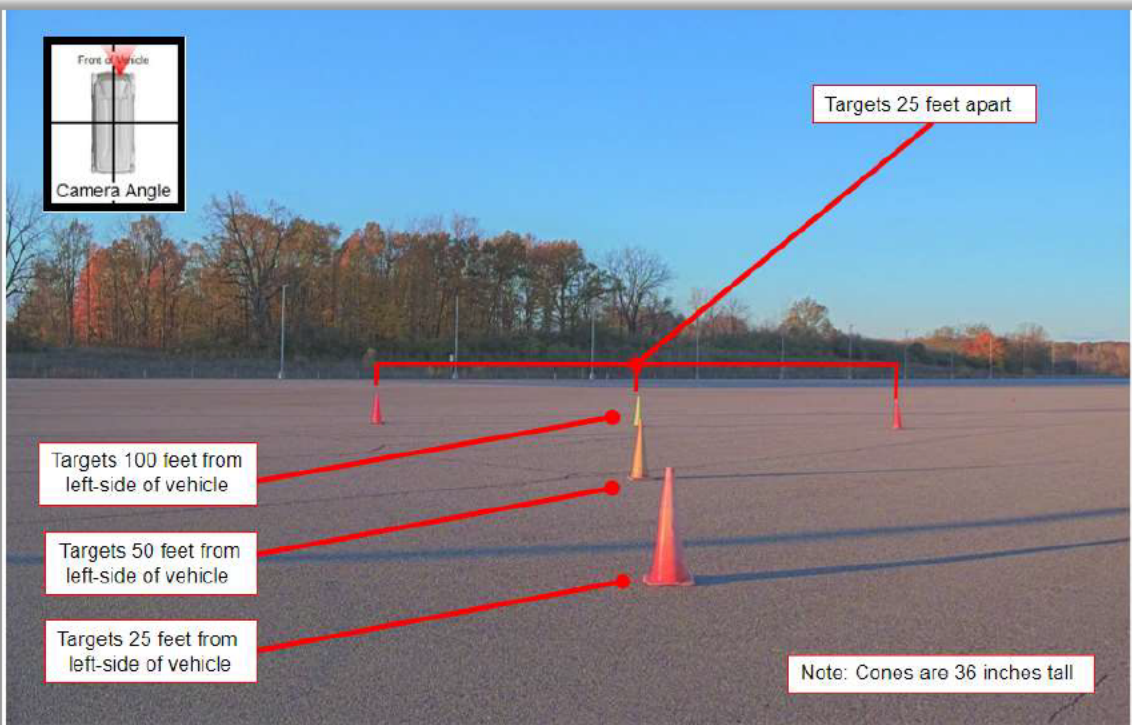
Figure C-17: Front Side Medium Resolution Camera Showing Forward Field of View
