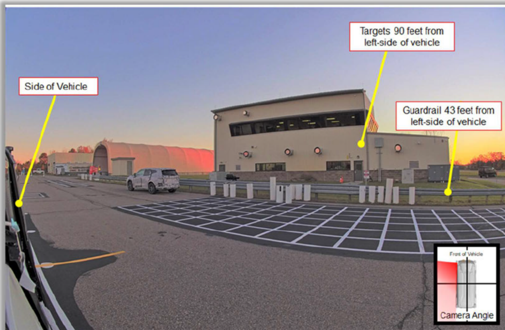
Figure C-21: Left Side Low Resolution Camera Showing Rear Left Side Field of View
