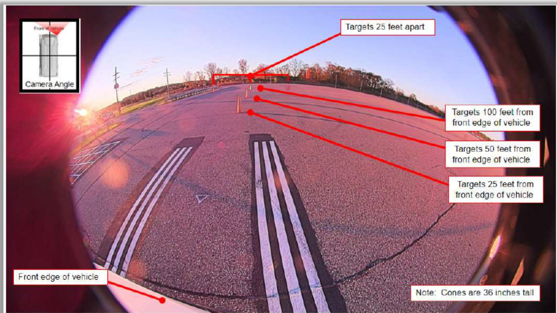
Figure C-15: Right/Front Side Surround View Camera Showing Forward Field of View
