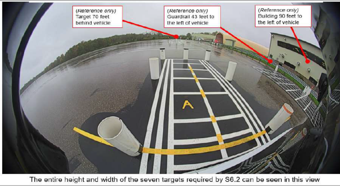
Figure 31: Origin’s Right Rear Surround Camera Showing FMVSS 111, S6.2 Rear Vision Grid
