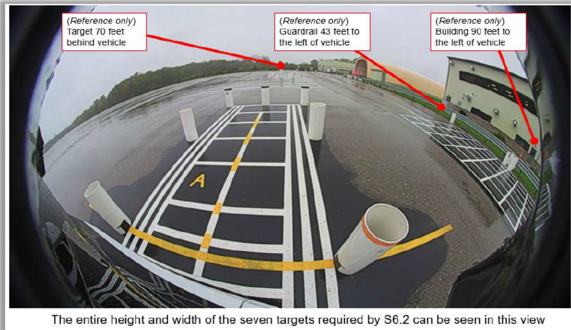
Figure 30: Origin's Left Rear Surround Camera Showing FMVSS 111, S6.2 Rear Vision Grid
