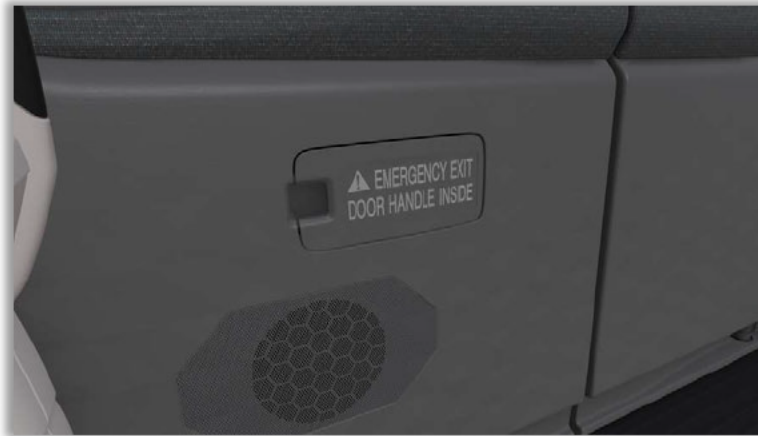
Figure 17: Emergency Exit Door Handle
