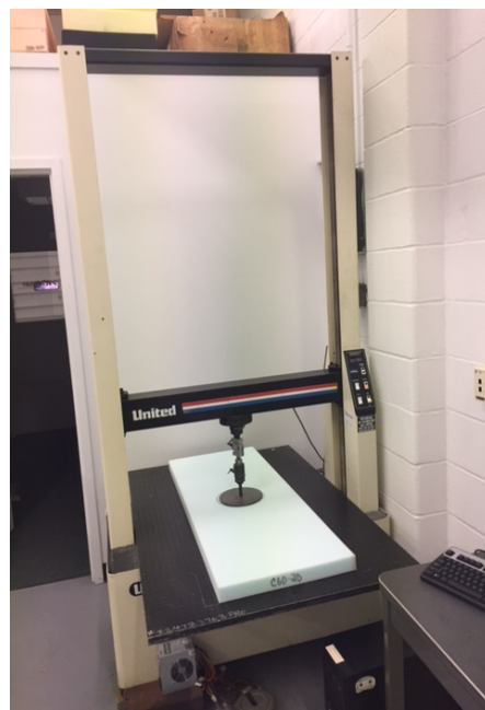
Figure 4-1. United Calibration Machine
