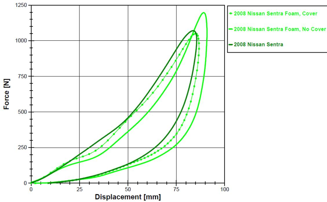
Figure 11. In-Vehicle and Out-of-Vehicle Nissan Sentra Results
