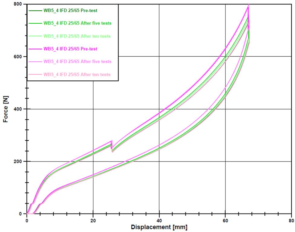
Figure 32. WB Foam 5 Force-Displacement Overlay for 25/65 Percent Testing
