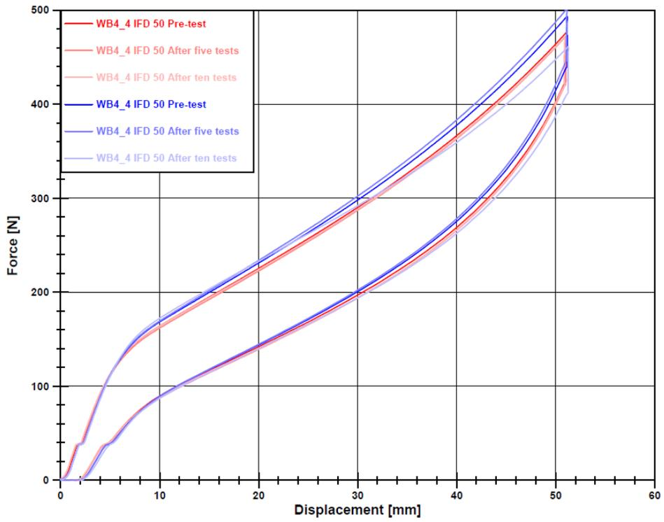
Figure 33. WB Foam 4 Force-Displacement Overlay for 50 Percent Testing
