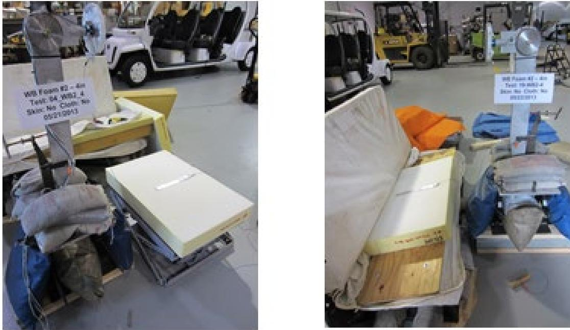
*Figure 18. Adjustable Table Versus FMVSS No. 213 Bench Set-up*
