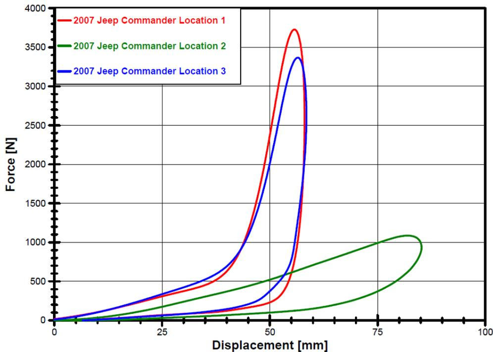
Figure 8. Dynamic Force-Displacement Curves for the 2007 Jeep Commander
