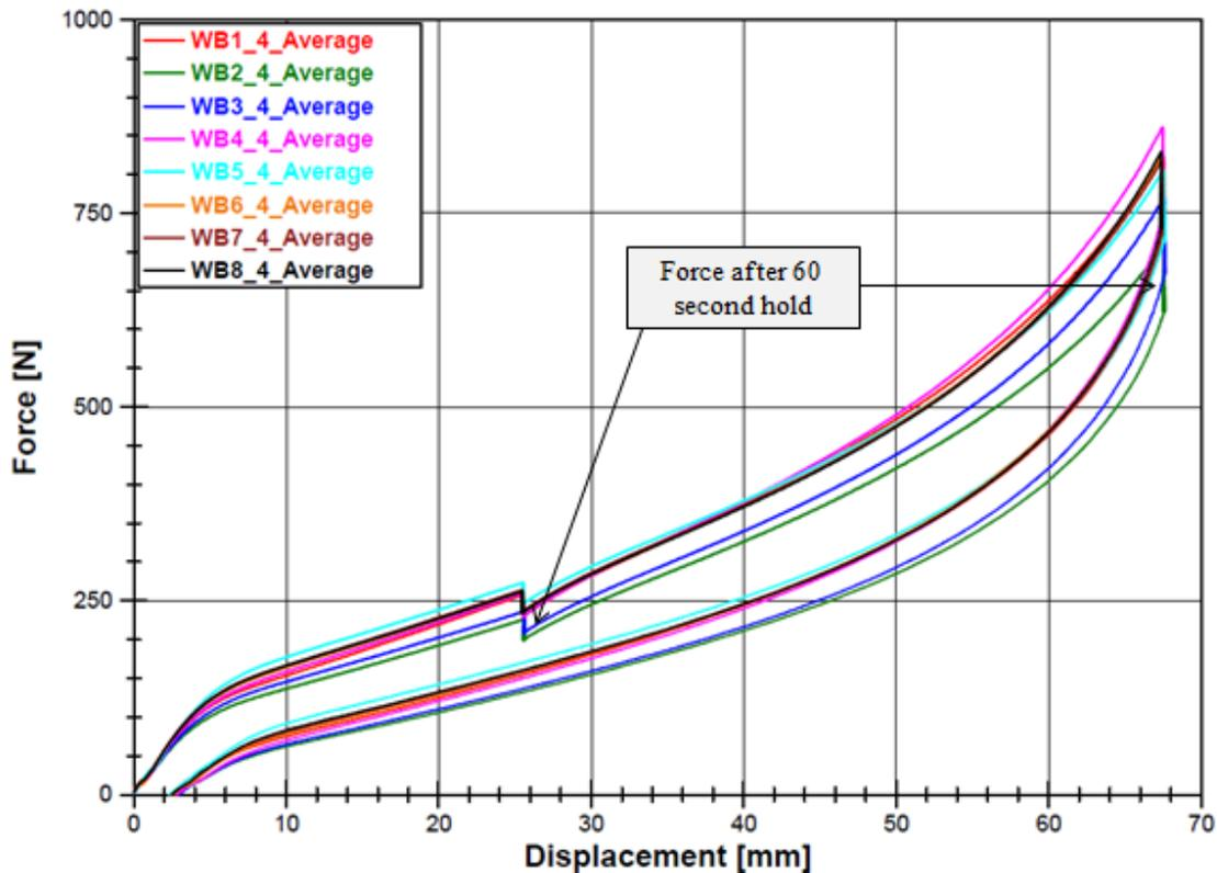
Figure 29. IFD Force-Displacement Curves for WB Foams 1 to 8
