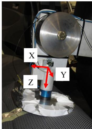
*Step 4: Attach the accelerometers, angular rate sensor, and load cell to the pendulum arm*
