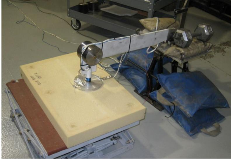
*Step 3: Measure the angle of the pendulum arm when it makes first contact with the foam*
