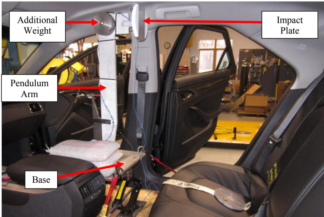
*Figure 5. Pendulum Impact Device*
