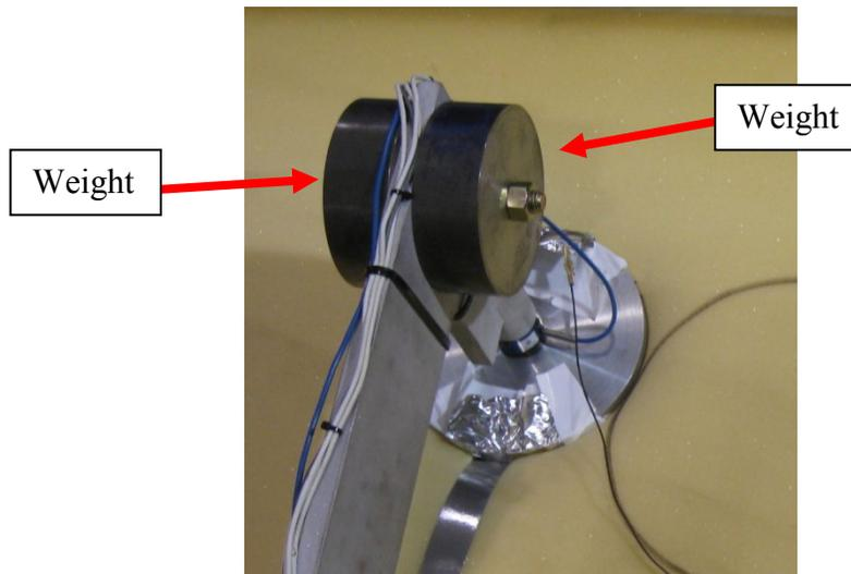
*Step 4: Add weight to the pendulum arm*
