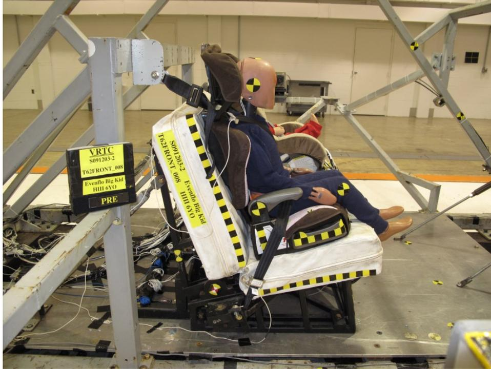
*Figure 4. FMVSS No. 213 Set-up*
