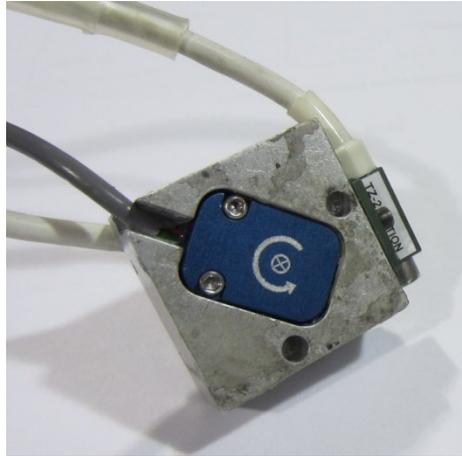
*Step 4: Attach an ARS and three accelerometers to the mounting block*
