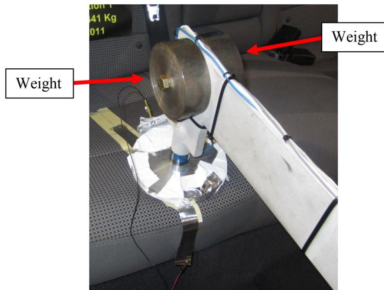
*Step 5: Add weight to the pendulum arm*
