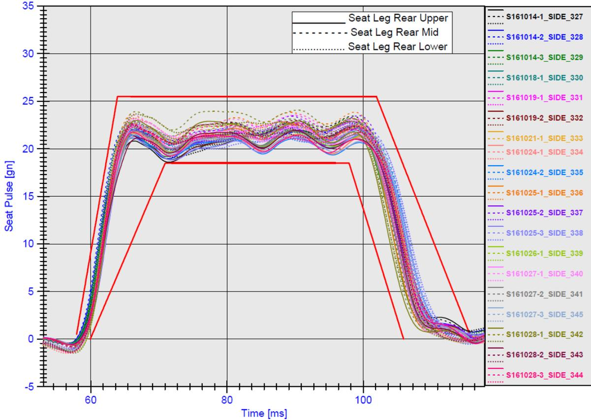
Figure 5. Sliding Seat Acceleration Results
