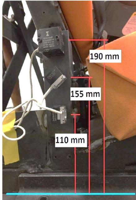
Figure 4. Accelerometer Placement on Rear Leg of Sliding Seat
