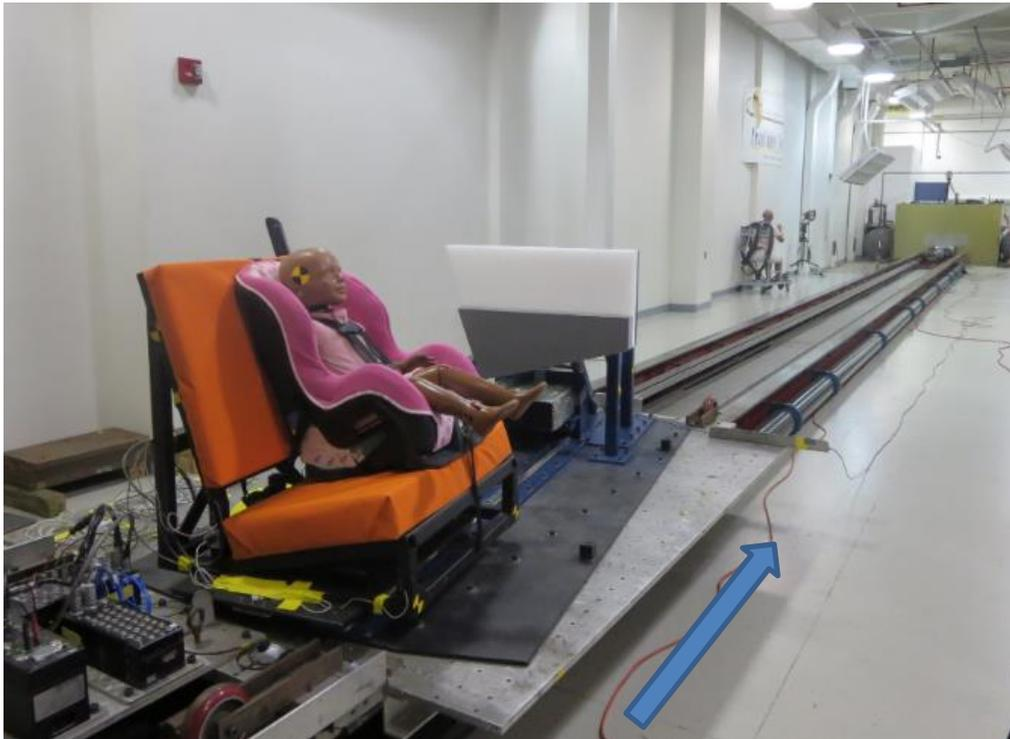
*Figure 2. KCS Deceleration Sled Set-up*
