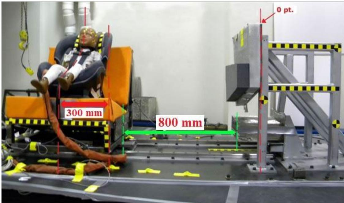
*Figure 9. Deceleration Set-up*
