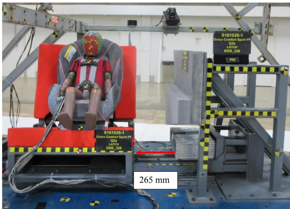
*Figure 8. Acceleration Set-up*
