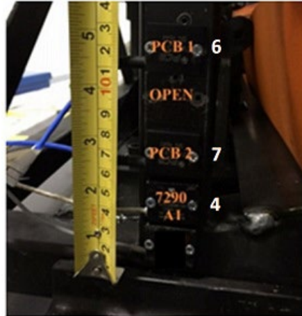
Figure B5: Configuration “D” - Outboard accelerometer placement
