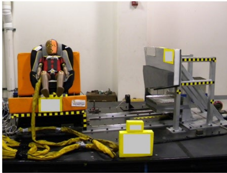
Figure C1: Front view of side impact fixture attached to the deceleration sled
