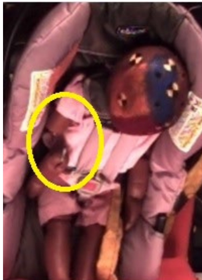
Figure 16: Screen shot from test DOT_SIDE_071 showing post impact elbow break
