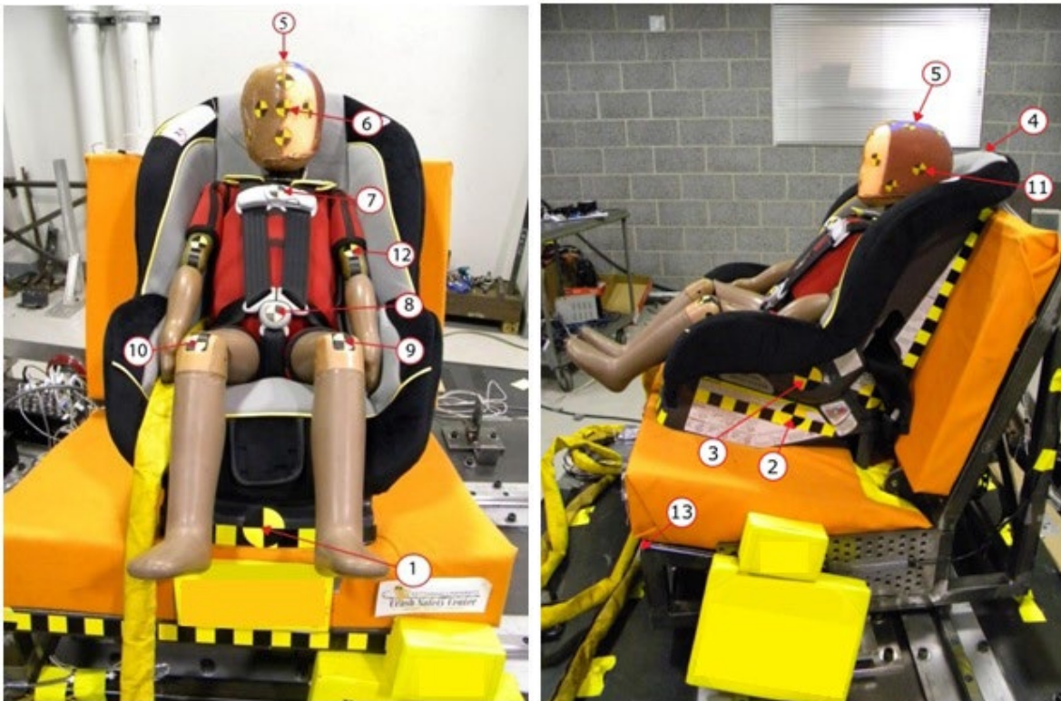
Figure C8: Layout of sample CMM measurement locations
