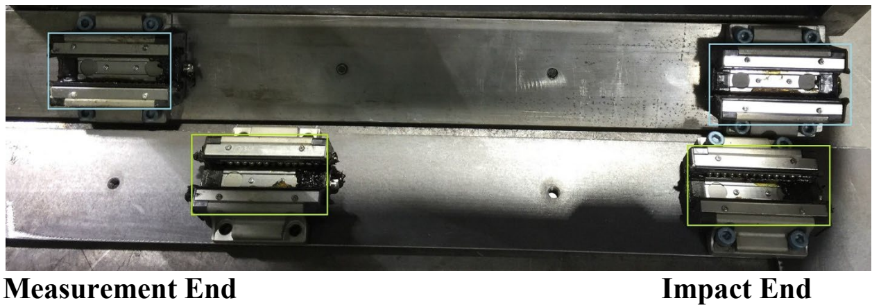
Figure A7: Side-by-side comparison of the KCS (blue) and design intent (green) bearing locations on the Rail Bearing Mount Plate (2921-396)
