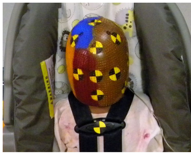
Figure C3: CRABI 12 heads prepared for testing with targets, copper mesh cover, and test chalk
