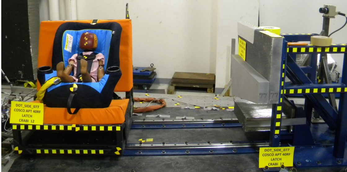
Figure 1: Side impact fixture attached to the deceleration sled
