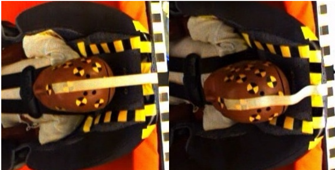
Figure 15: Overhead still photos from high-speed video depicting maximum forward and rearward movement of taped ATD head
