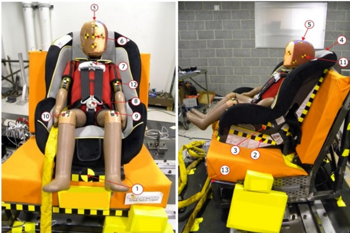
Figure B9: Layout of sample CMM measurement locations
