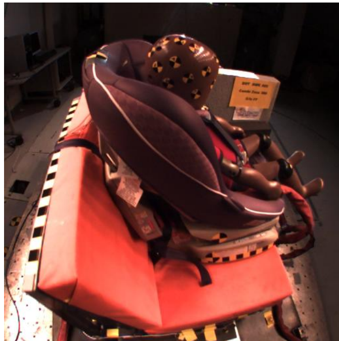
Figure 13: Inline views of Q3s left at time of impact of CRS with the door foam from Phase I testing
