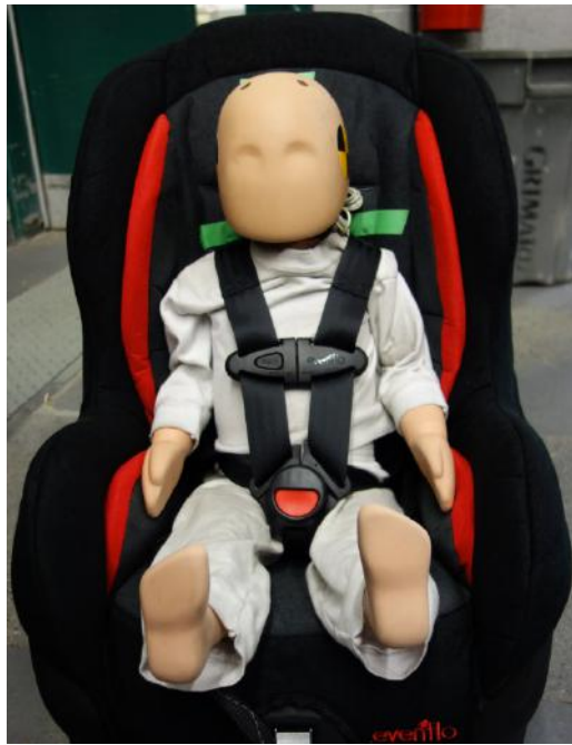
Figure 10: Photograph of the dummy positioned in the child restraint system showing the three marker positions.
