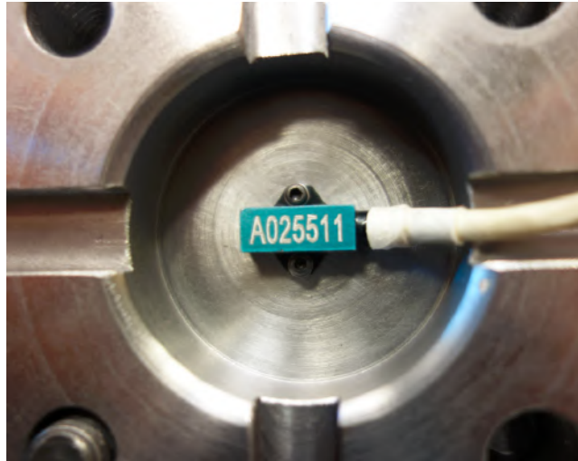
Figure 7: Photograph of the accelerometer fastened inside the headform.
