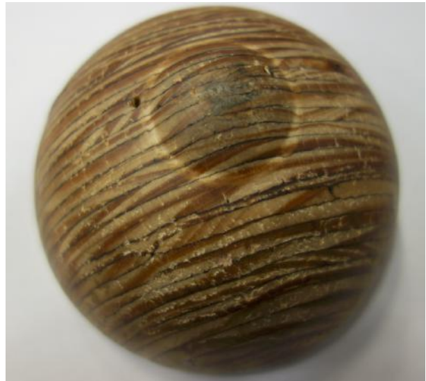
Figure 3: Photograph of the solid wooden hemisphere of the headform (top view).
