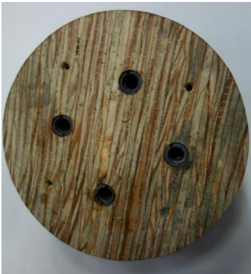
Figure 4: Photograph of the solid wooden hemisphere of the headform (bottom view).
