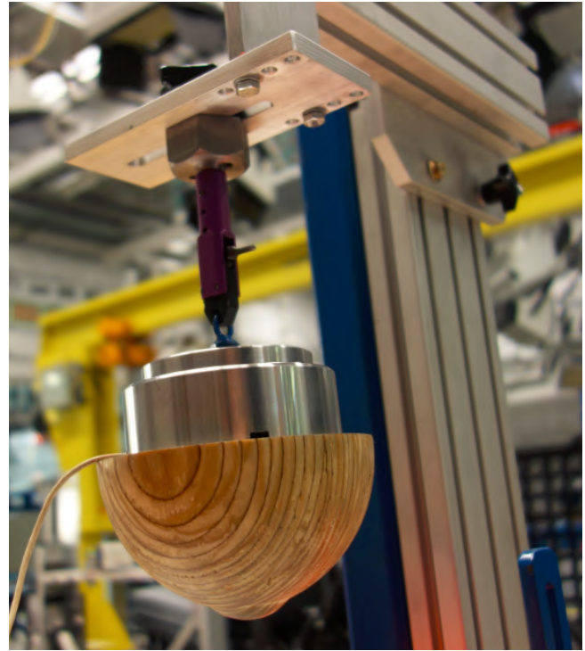
Figure 9: Photograph of the apparatus which holds up the headform on the drop-test structure.
