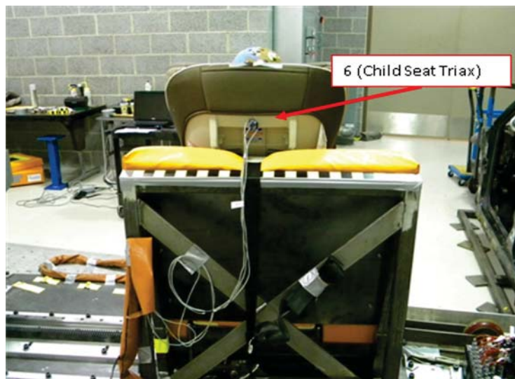
Figure 13: Location of accelerometers on test fixture and child restraint system
