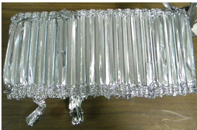
Figure 22: Post-test aluminum honeycomb block showing the irregular profile
