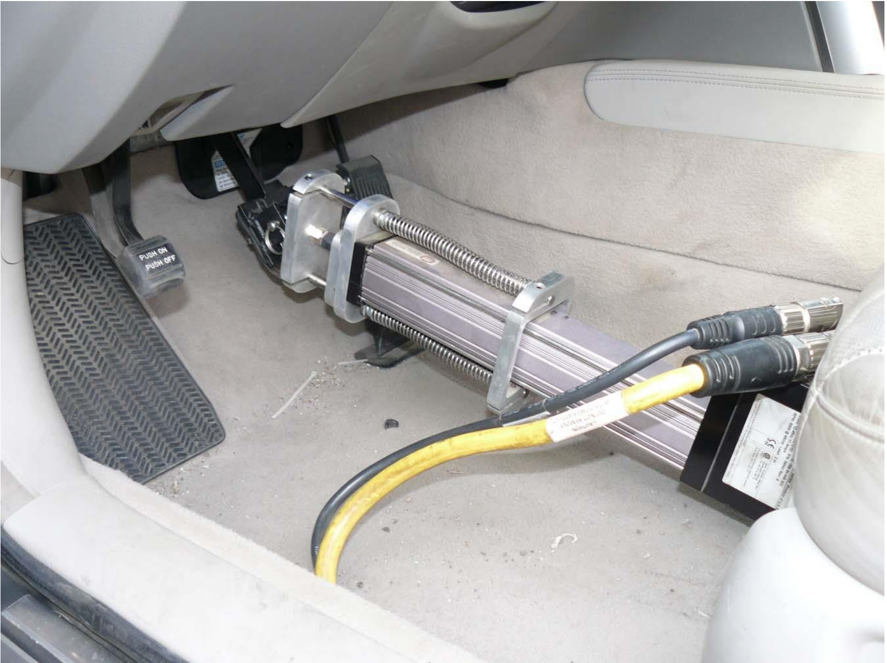
Figure A14. Brake Actuator Installed in POV System
