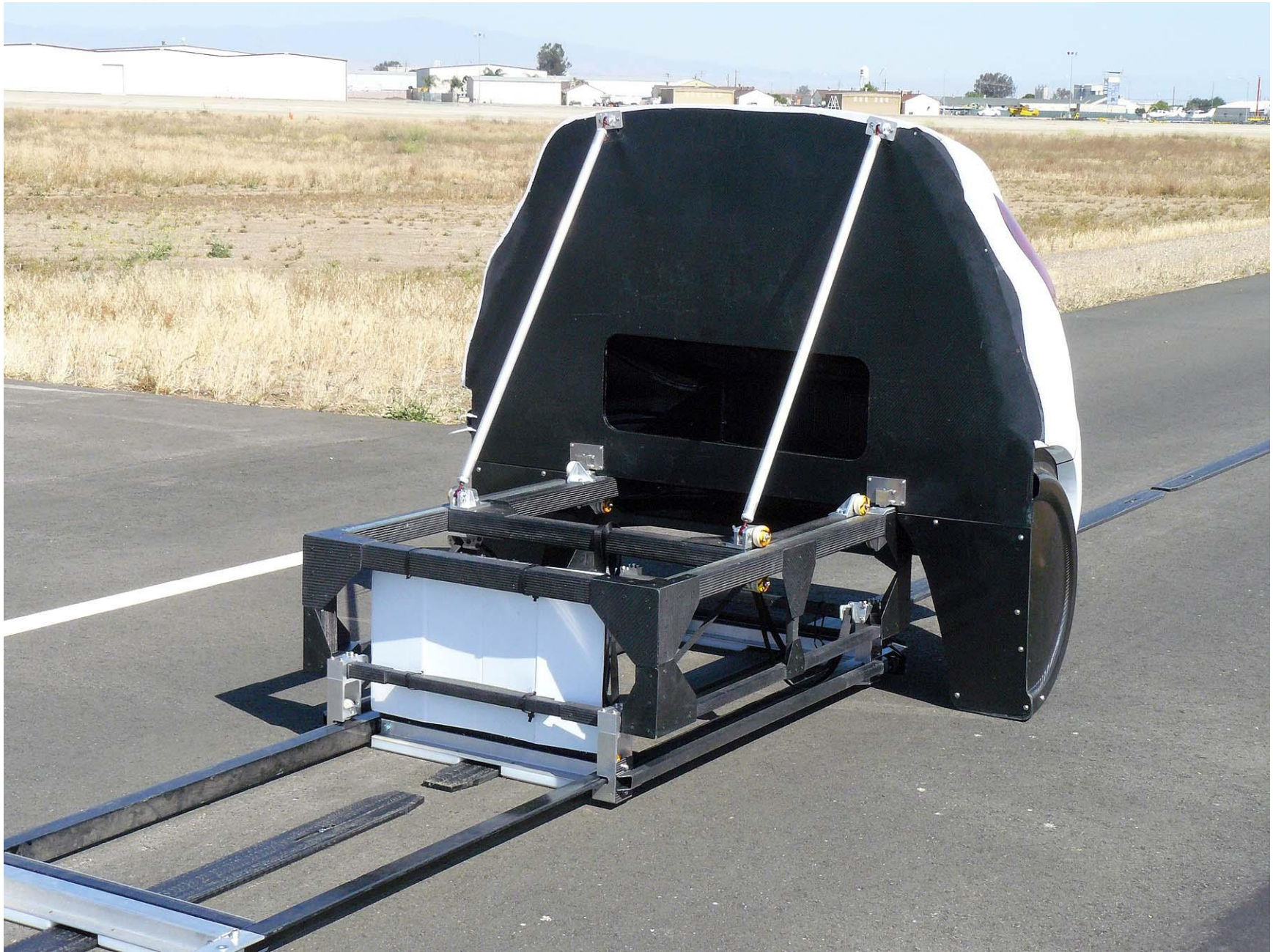
Figure A7. Load Frame/Slider of SSV
