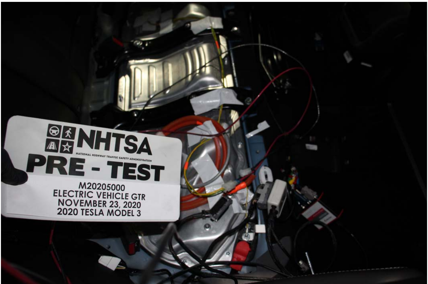
Photo No. 026 - Overcurrent Breakout Harness
