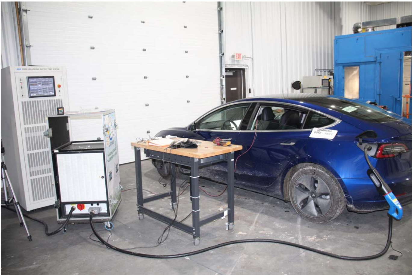
Photo No. 027 - Overcurrent Test Setup
