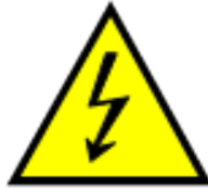
Figure 1- Marking of High Voltage Equipment
