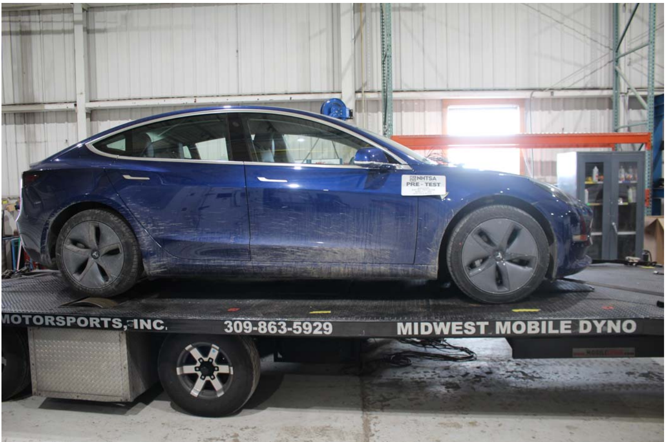
Photo No. 024 - Over-temperature Test Setup
