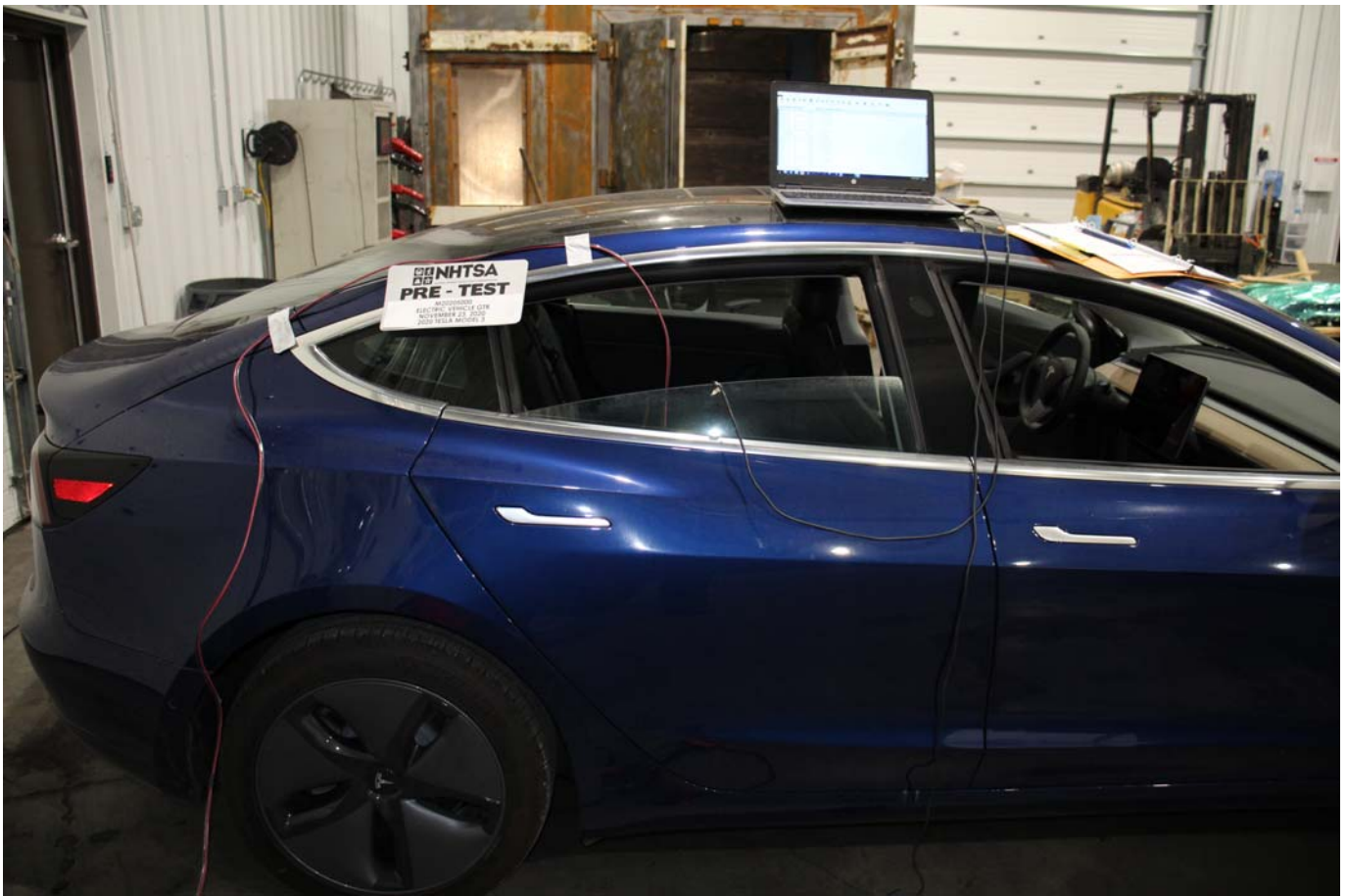
Photo No. 021 - Over-discharge Test Setup
