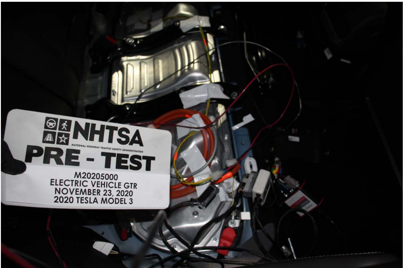
Photo No. 020 - Over-discharge Breakout Harness
