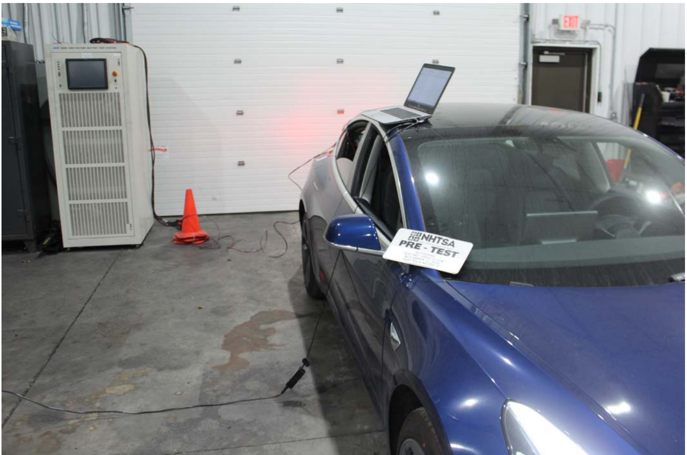
Photo No. 018 - Overcharge Test Setup
