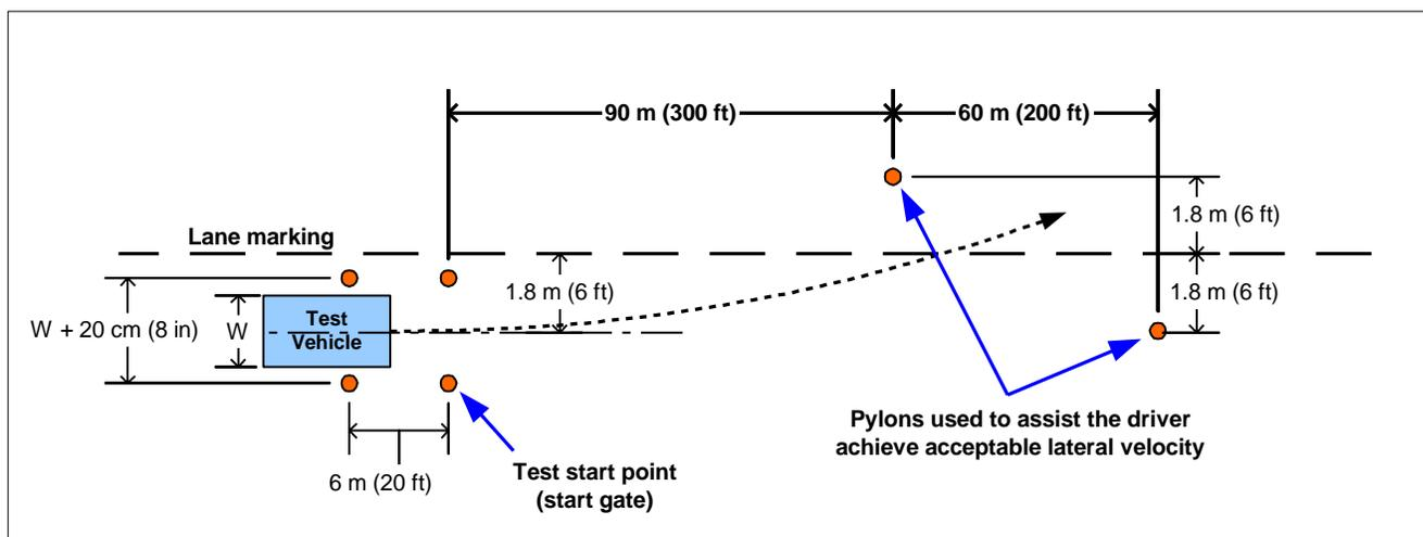
Figure 1. Position of Cones Used to Assist Driver
