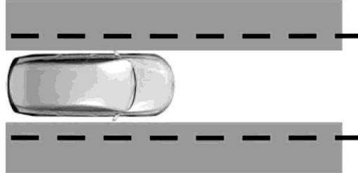
The lane keeping system aids you when an unintentional lane departure occurs. The system provides a small steering input to move the vehicle towards the center of the lane.
