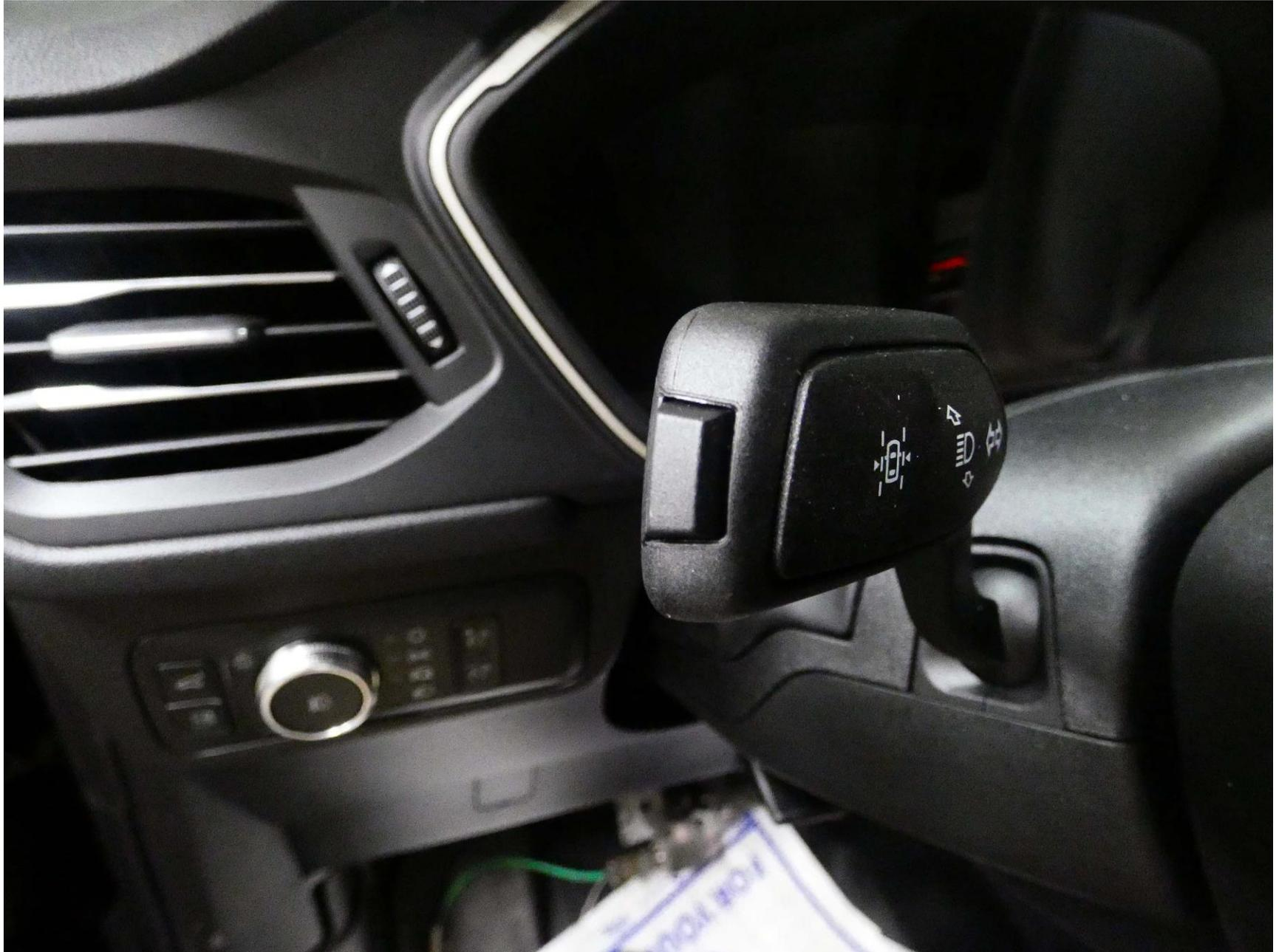
Figure A10. LDW System On/Off Button
