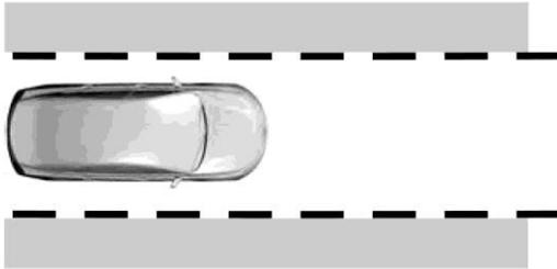
When in alert mode, the lane keeping system alerts you by vibrating the steering wheel. The intensity of the vibration is set through the lane keeping system menu.
