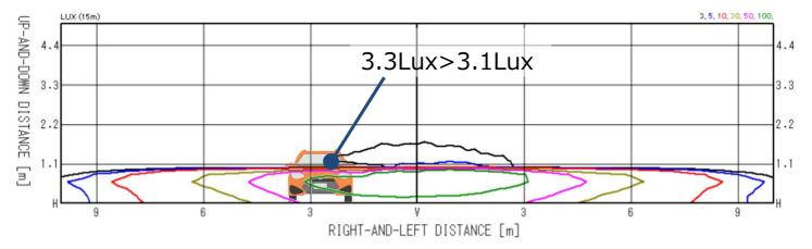
There is a possibility that a low-beam alone (with ADB turned off) does not comply with the ADB glare requirement in Table XXI.
