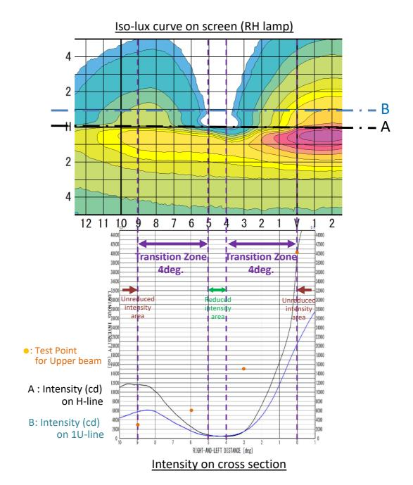
This ADB needs 4-degree Transition Zone for complying with the photometric requirement of the unreduced intensity area (40,000 cd min. at HV).
