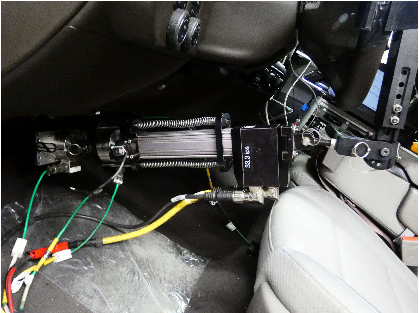
Figure A13. Brake Actuator Installed in Subject Vehicle A-15
