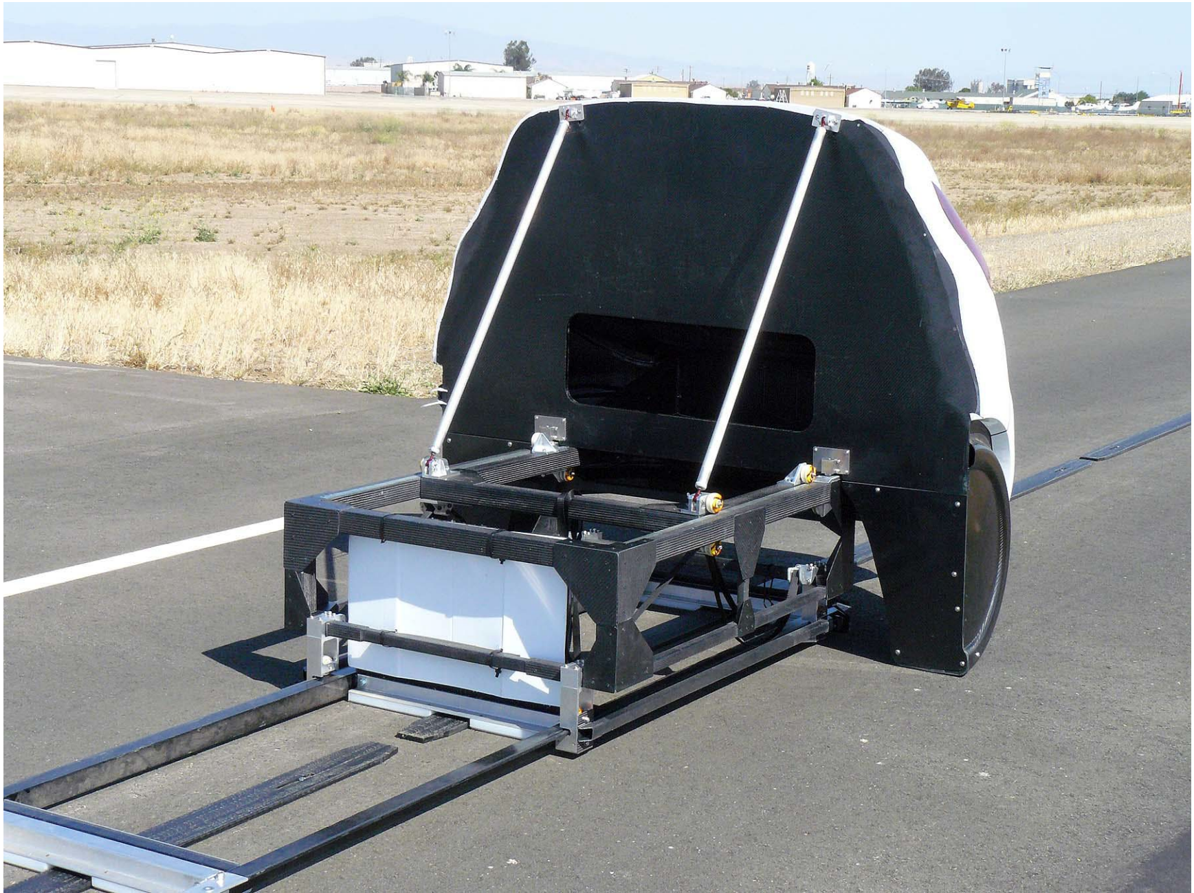
Figure A7. Load Frame/Slider of SSV
