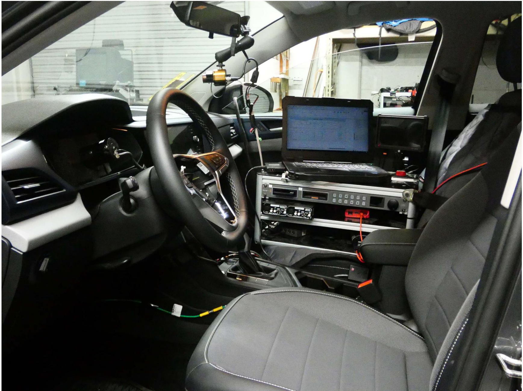
Figure A12. Computer Installed in Subject Vehicle
