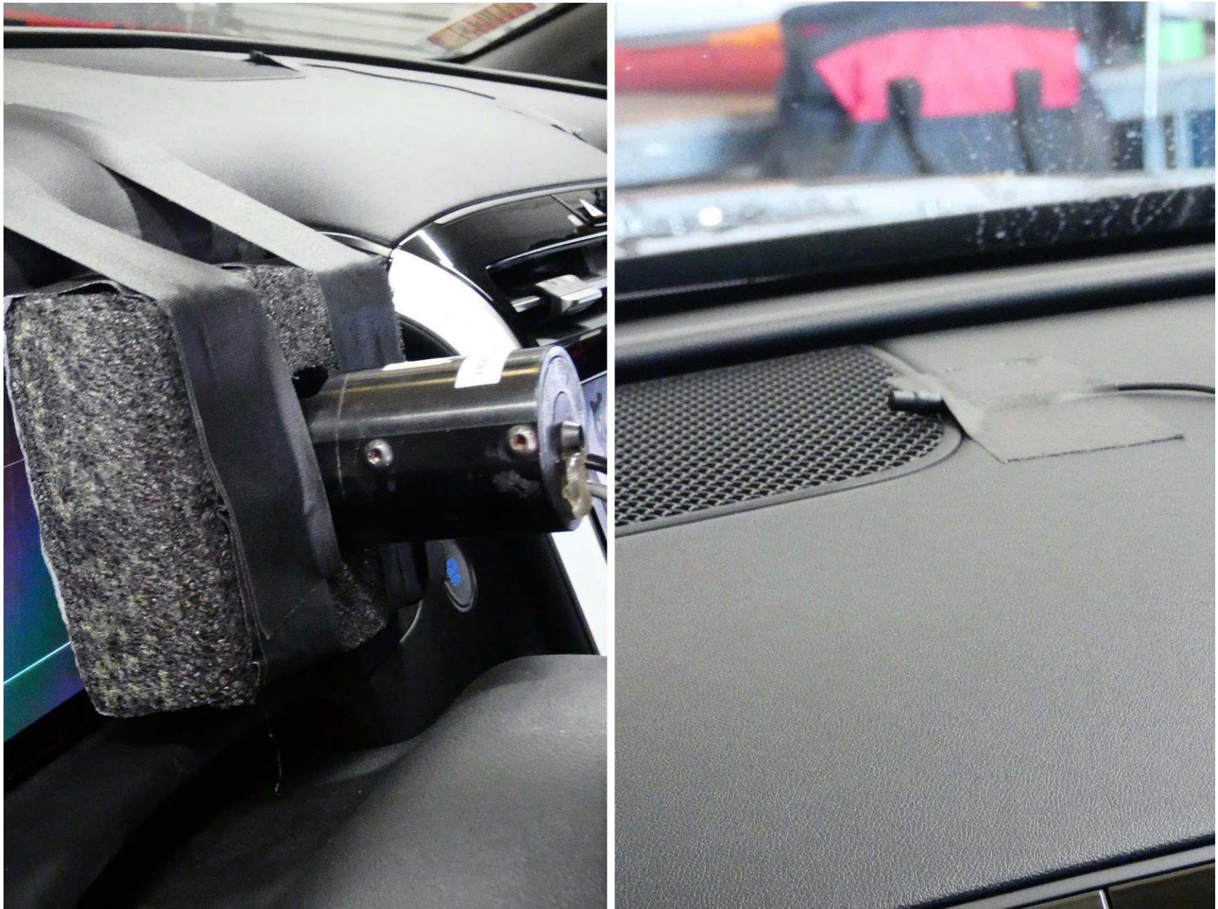
Figure A11. Sensor for Detecting Auditory and Visual Alerts
