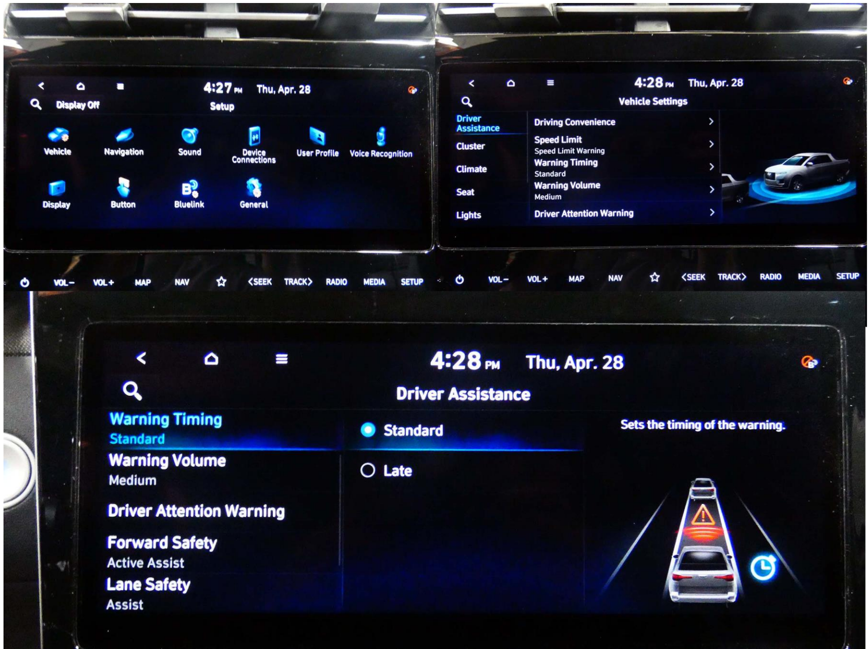
Figure A14. AEB System Warning Timing Setup
