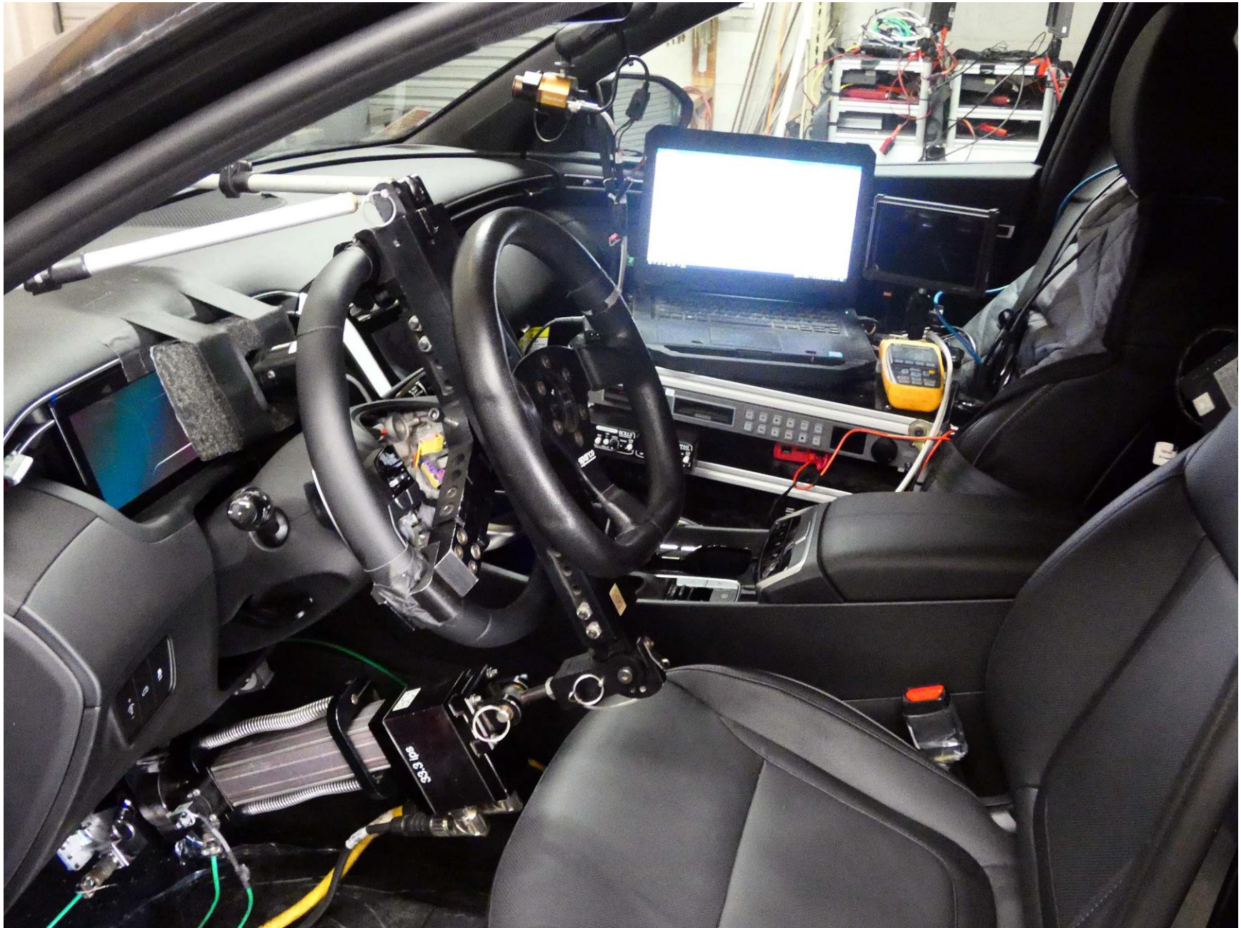
Figure A12. Computer Installed in Subject Vehicle
