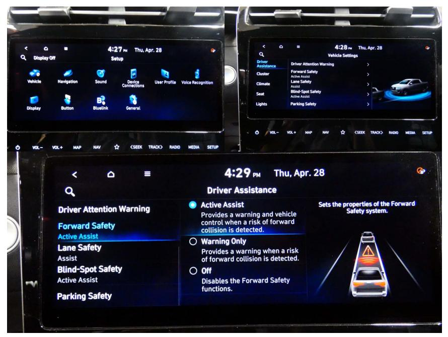
Figure A15. AEB System On/Off
