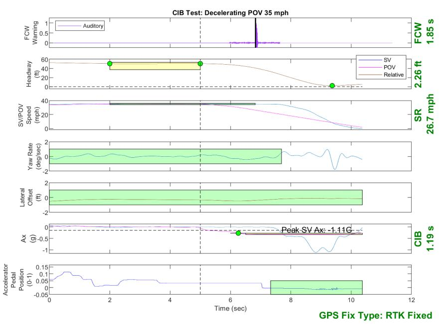
Figure D4. Example Time History for Decelerating POV 35, Passing
