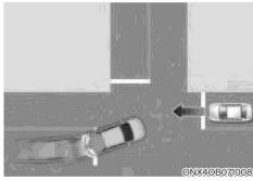
The Junction Turning function can help avoid a collision with an oncoming vehicle when attempting to make a left hand turn at an intersection. If the function detects that a collision is imminent, a warning message occurs and in certain cases, emergency braking may be applied.
