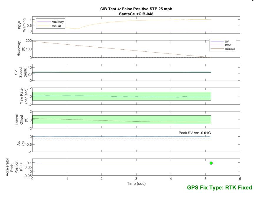
Figure D44. Time History for CIB Run 48, Test 4 - False Positive STP, 25 mph
