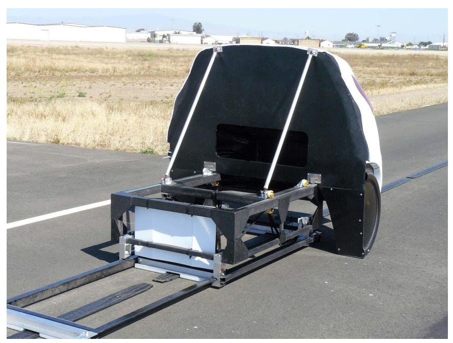
Figure A7. Load Frame/Slider of SSV
