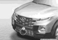
[1]: Front view camera,[2]: Front radarRefer to the picture above for the detailed location of the detecting
