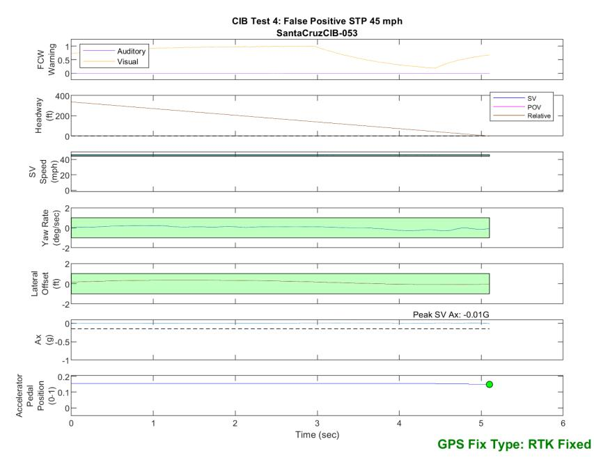
Figure D48. Time History for CIB Run 53, Test 4 - False Positive STP, 45 mph
