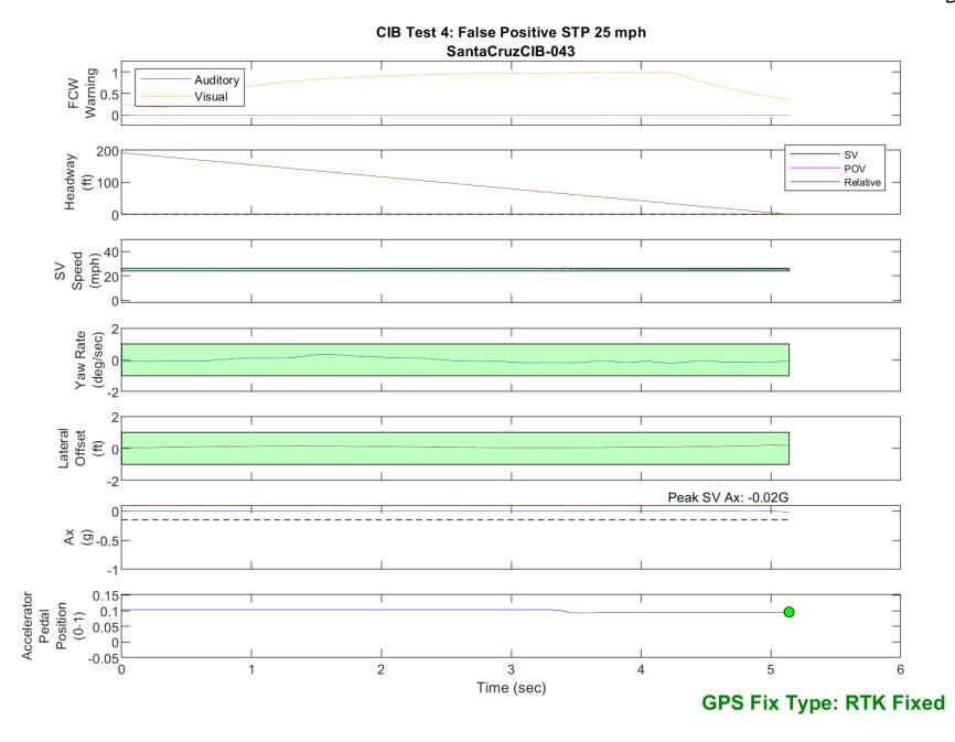
Figure D39. Time History for CIB Run 43, Test 4 - False Positive STP, 25 mph
