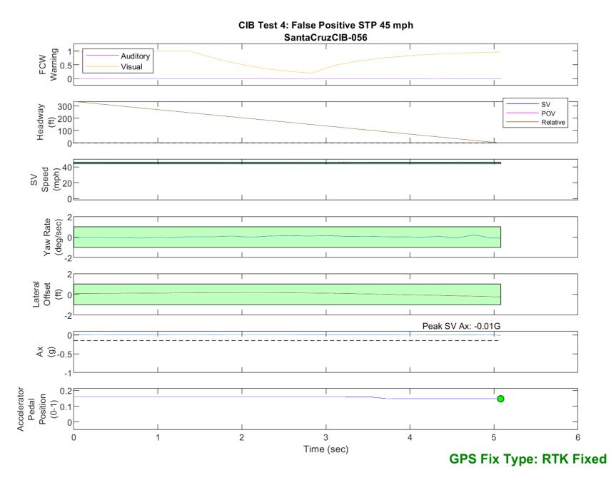
Figure D51. Time History for CIB Run 56, Test 4 - False Positive STP, 45 mph
