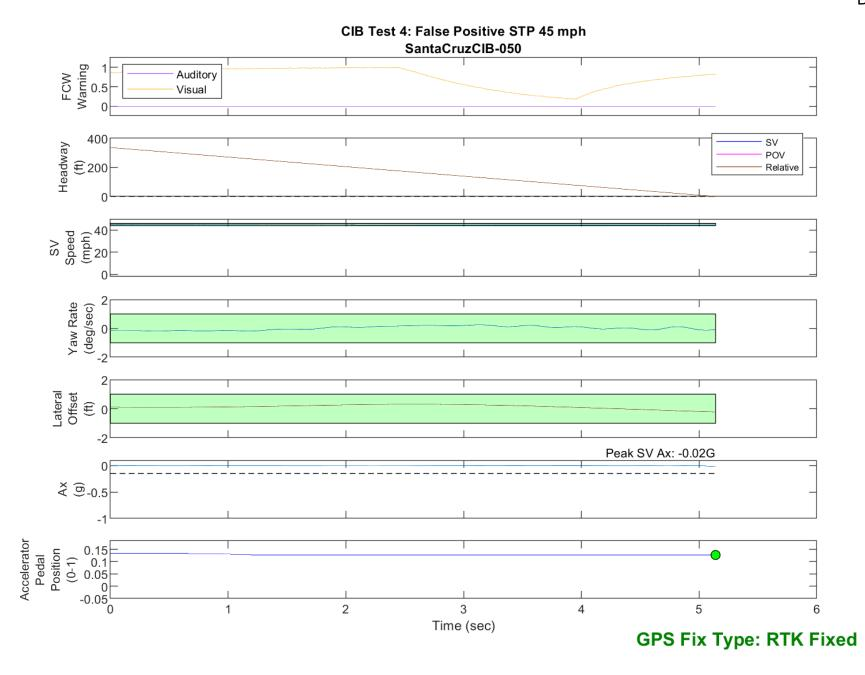
Figure D45. Time History for CIB Run 50, Test 4 - False Positive STP, 45 mph
