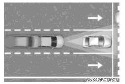
Forward Collision Avoidance Assist is designed to help detect and monitor a vehicle on the roadway ahead or help detect if a pedestrian or cyclist is in the roadway. Forward Collision Avoidance Assist will warn the driver with an audible warning and a message in the LCD cluster if it determines that a collision is imminent. In certain cases, emergency braking may be applied.
