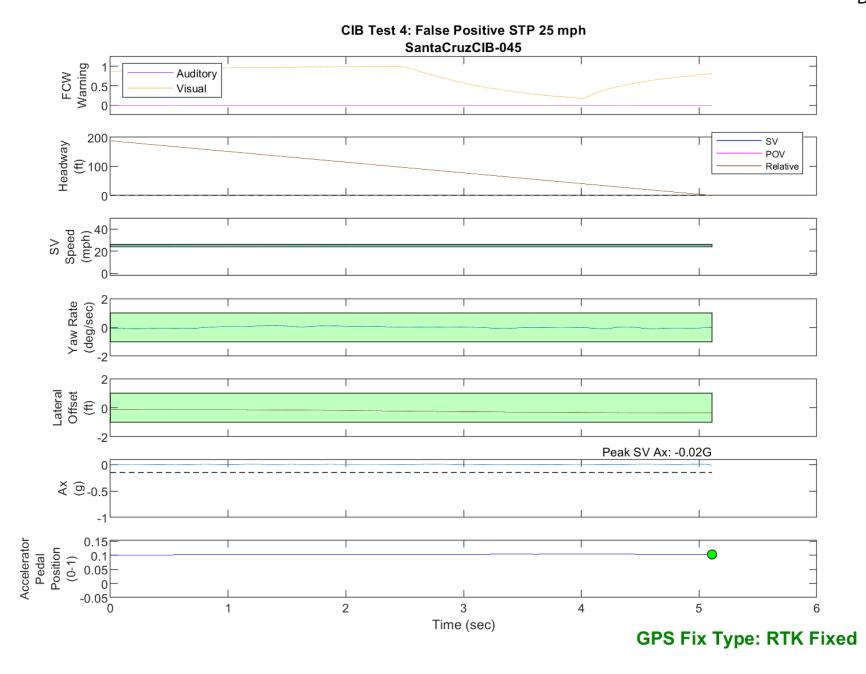
Figure D41. Time History for CIB Run 45, Test 4 - False Positive STP, 25 mph
