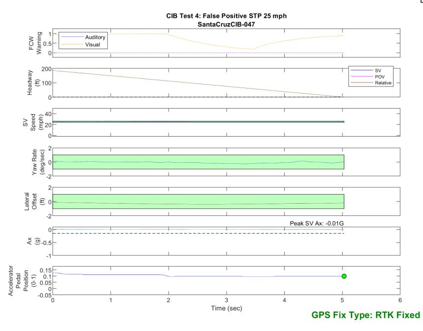
Figure D43. Time History for CIB Run 47, Test 4 - False Positive STP, 25 mph
