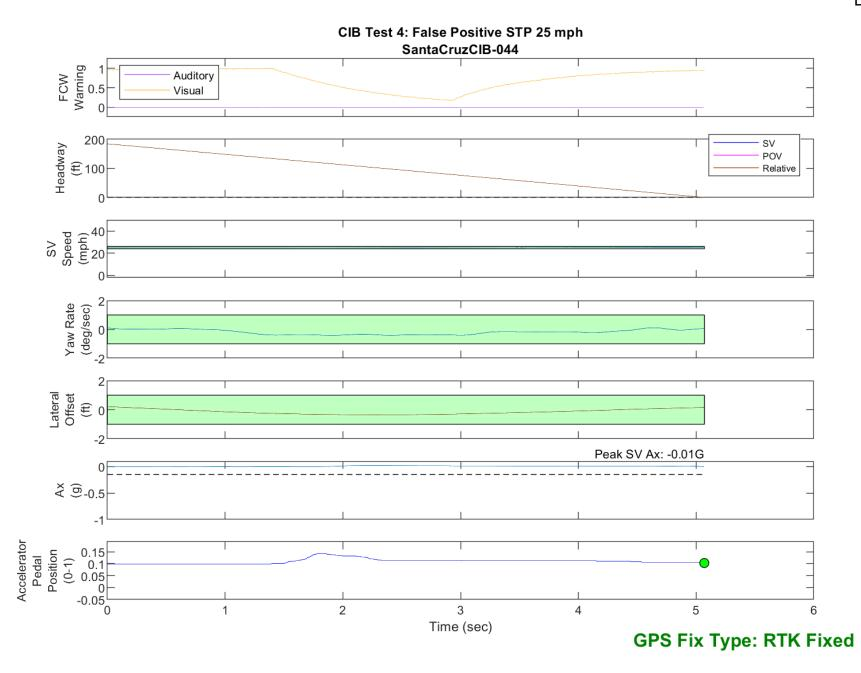
Figure D40. Time History for CIB Run 44, Test 4 - False Positive STP, 25 mph
