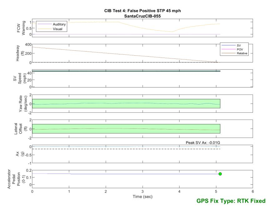
Figure D50. Time History for CIB Run 55, Test 4 - False Positive STP, 45 mph
