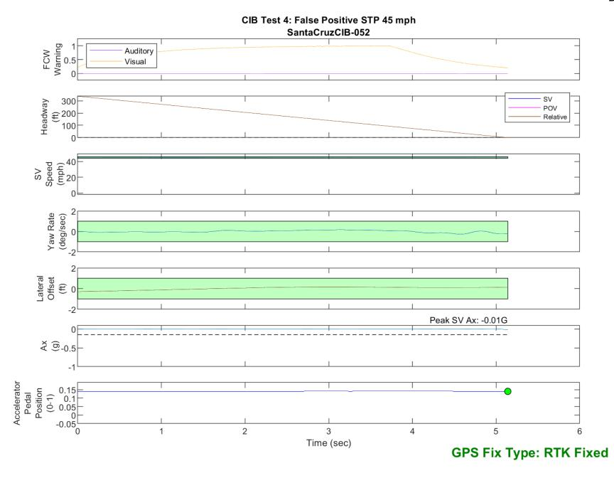
Figure D47. Time History for CIB Run 52, Test 4 - False Positive STP, 45 mph
