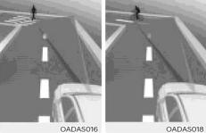
Forward Collision-Avoidance Assist may not detect other vehicles, pedestrians or cyclists in front of you on curved roads adversely affecting the performance of the sensors. This may result in no warning or braking assist when necessary.
