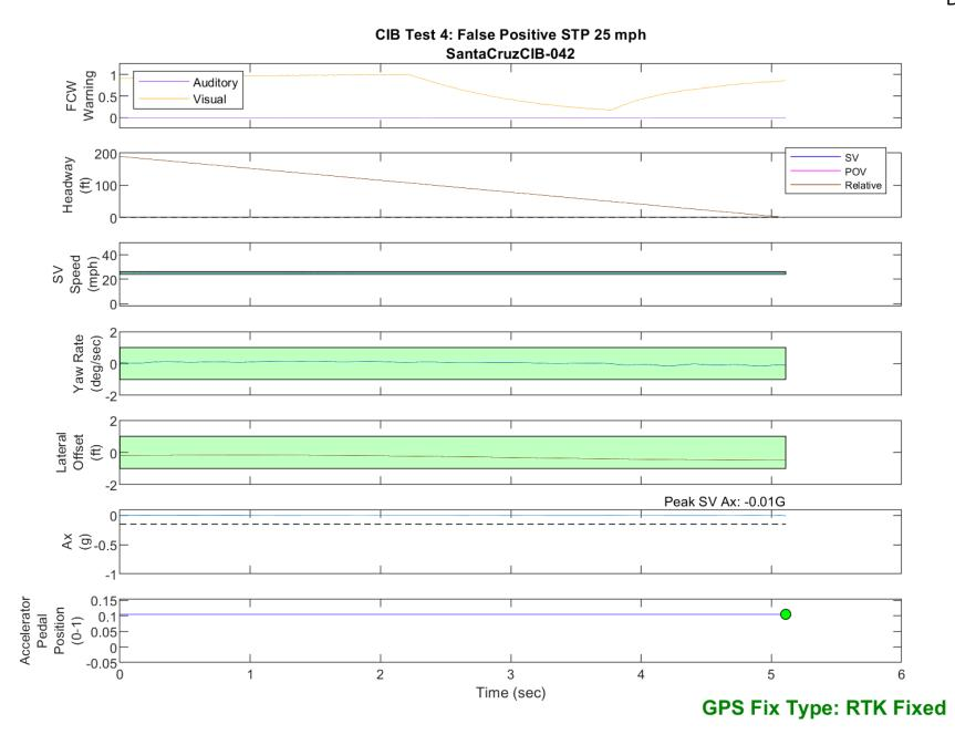
Figure D38. Time History for CIB Run 42, Test 4 - False Positive STP, 25 mph
