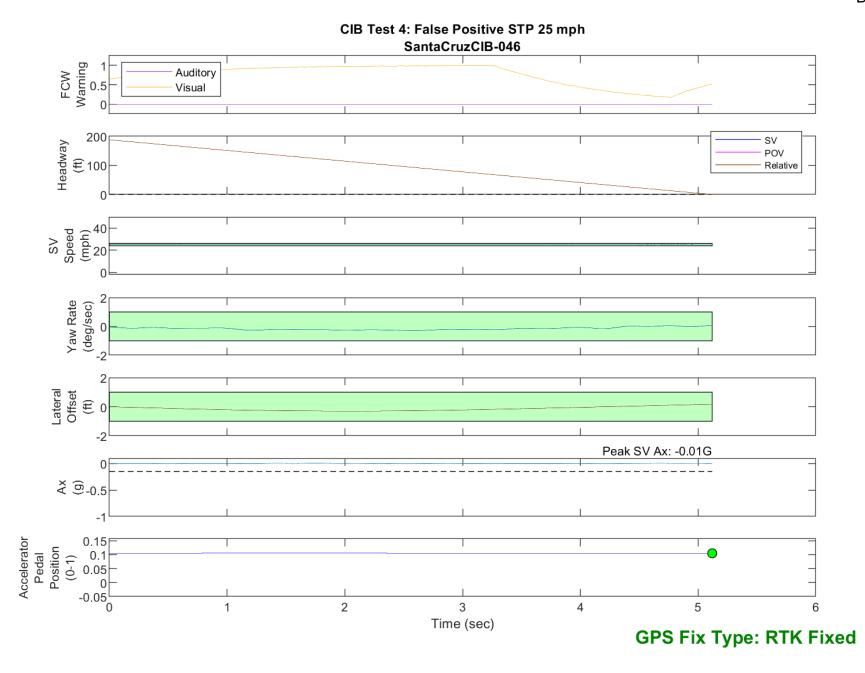
Figure D42. Time History for CIB Run 46, Test 4 - False Positive STP, 25 mph
