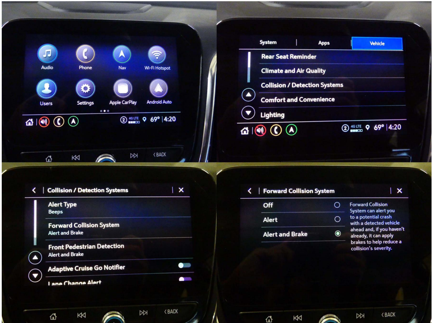
Figure A15. AEB System Setup Menus
