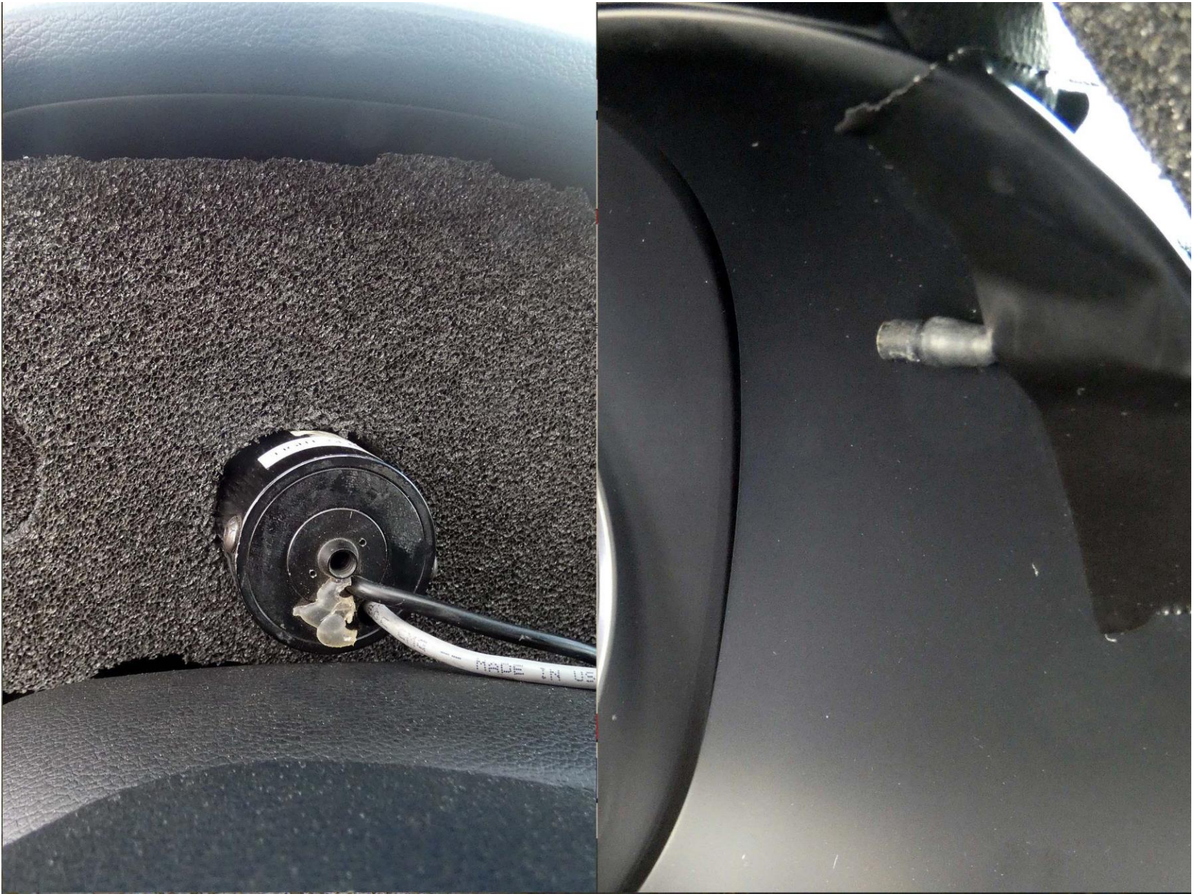
Figure A8. Sensors for Detecting Visual and Auditory Alerts
