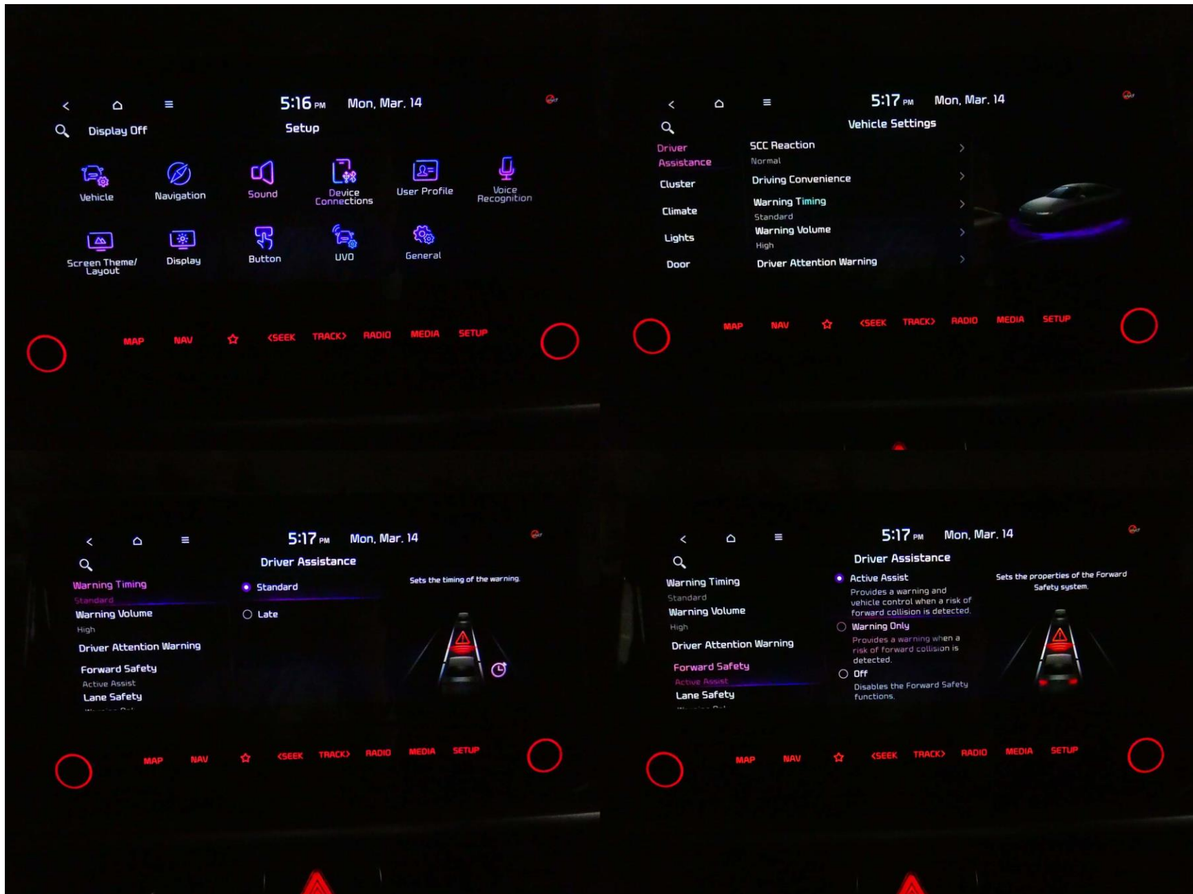
Figure A15. AEB System Setup Menus
