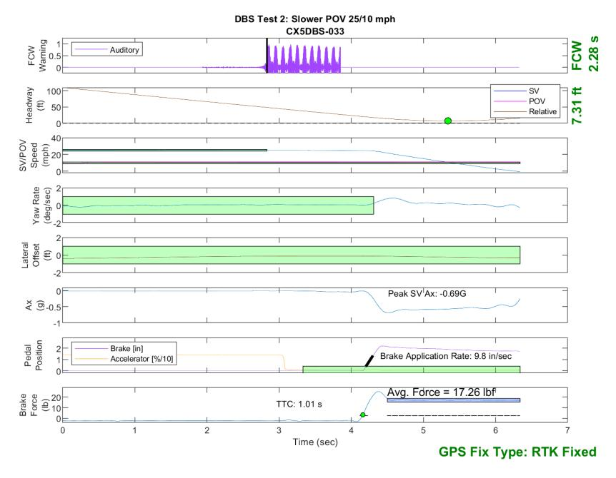
Figure E25. Time History for DBS Run 33, Test 2 - Slower Moving POV 25/10 mph
