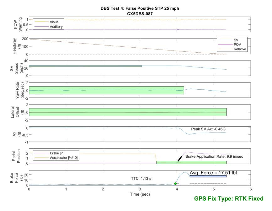
Figure E59. Time History for DBS Run 87, Test 4 - False Positive STP 25 mph
