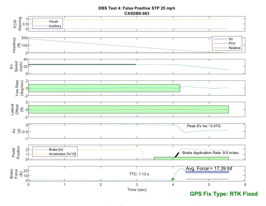
Figure E56. Time History for DBS Run 83, Test 4 - False Positive STP 25 mph
