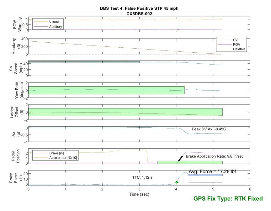
Figure E63. Time History for DBS Run 92, Test 4 - False Positive STP 45 mph
