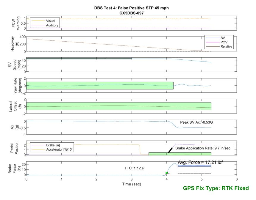
Figure E67. Time History for DBS Run 97, Test 4 - False Positive STP 45 mph
