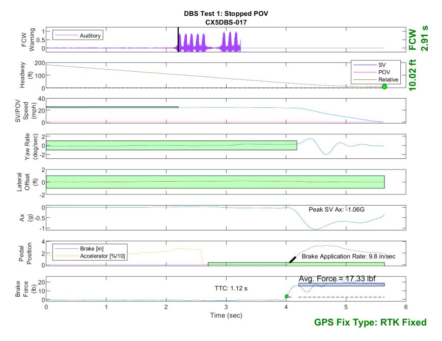
Figure E13. Time History for DBS Run 17, Test 1 - Stopped POV
