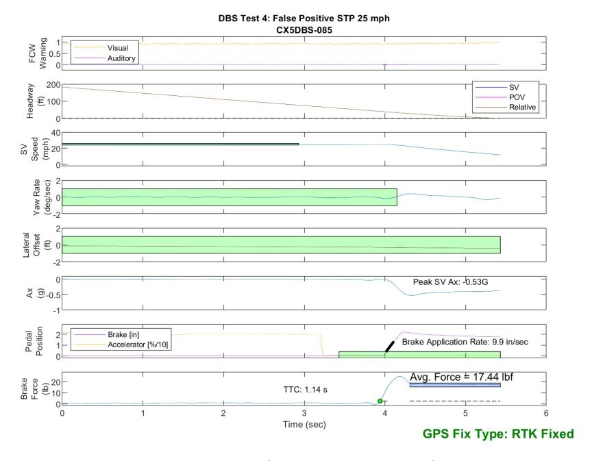
Figure E58. Time History for DBS Run 85, Test 4 - False Positive STP 25 mph
