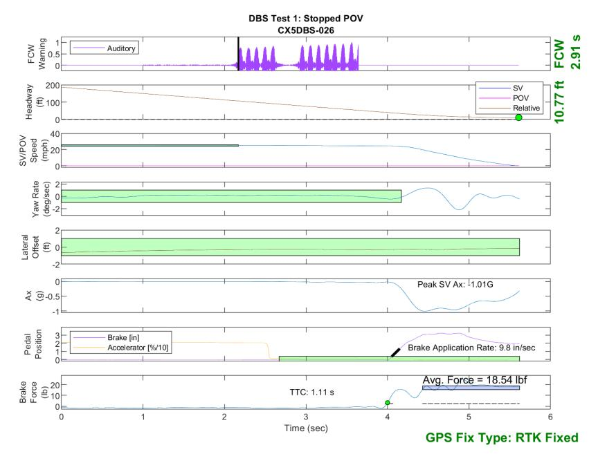
Figure E19. Time History for DBS Run 26, Test 1 - Stopped POV
