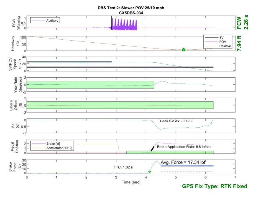
Figure E26. Time History for DBS Run 34, Test 2 - Slower Moving POV 25/10 mph
