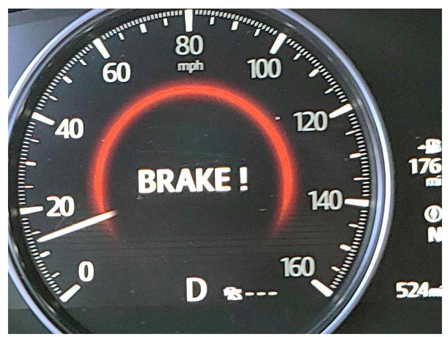
Figure A17. Visual Alert in Instrument Panel A-19
