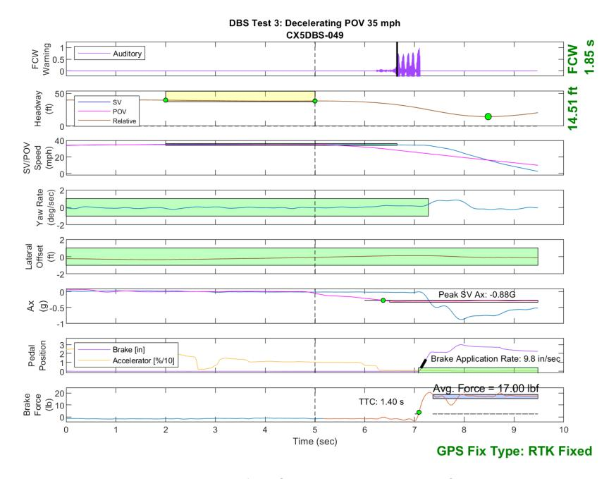
Figure E36. Time History for DBS Run 49, Test 3 - Decelerating POV 35 mph
