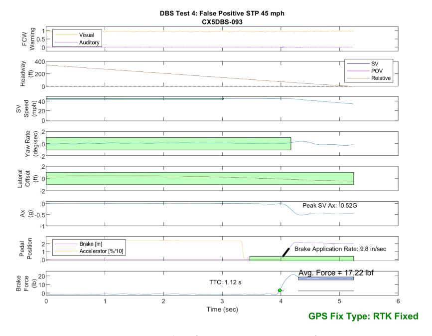
Figure E64. Time History for DBS Run 93, Test 4 - False Positive STP 45 mph
