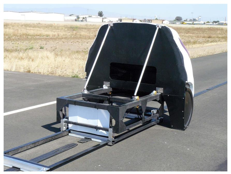
Figure A7. Load Frame/Slider of SSV A-9
