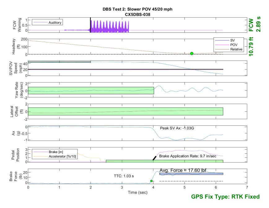
Figure E28. Time History for DBS Run 38, Test 2 - Slower Moving POV 45/20 mph
