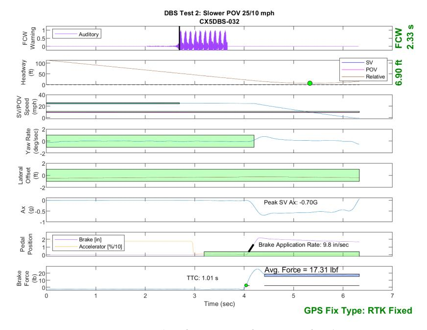
Figure E24. Time History for DBS Run 32, Test 2 - Slower Moving POV 25/10 mph
