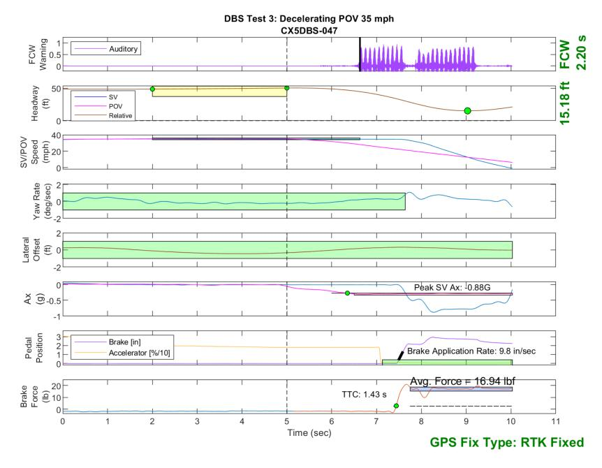
Figure E34. Time History for DBS Run 47, Test 3 - Decelerating POV 35 mph
