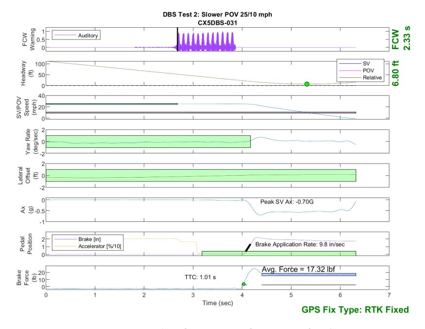
Figure E23. Time History for DBS Run 31, Test 2 - Slower Moving POV 25/10 mph
