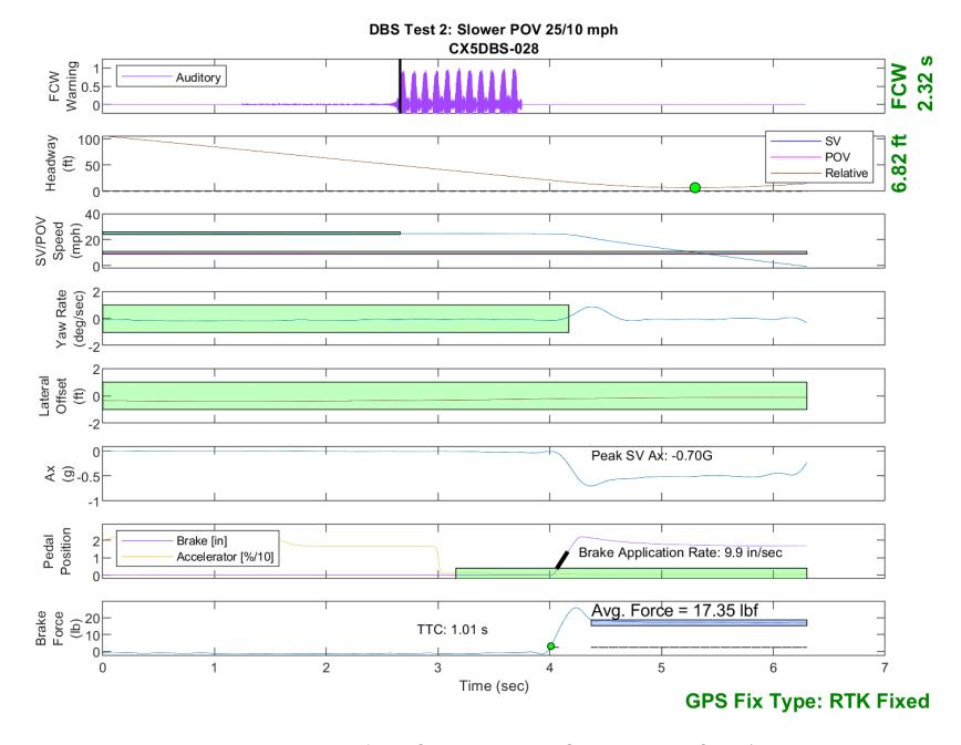
Figure E20. Time History for DBS Run 28, Test 2 - Slower Moving POV 25/10 mph
