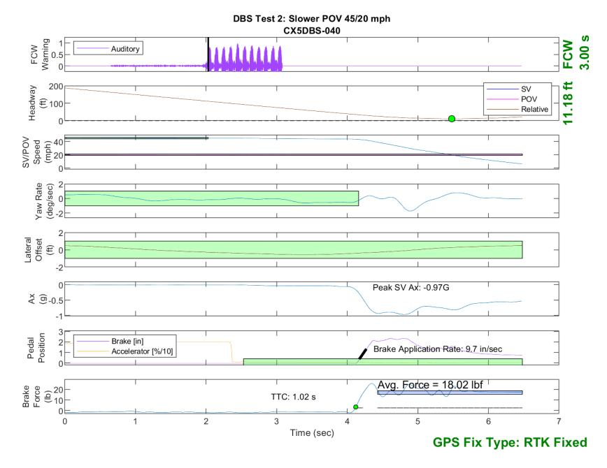
Figure E30. Time History for DBS Run 40, Test 2 - Slower Moving POV 45/20 mph
