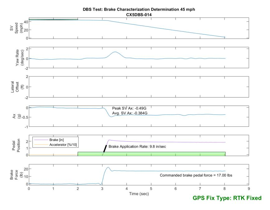
Figure E81. Time History for DBS Run 14, Brake Characterization Determination, Hybrid Mode, 45 mph
