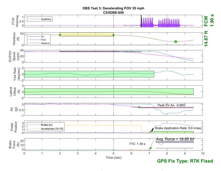
Figure E37. Time History for DBS Run 50, Test 3 - Decelerating POV 35 mph
