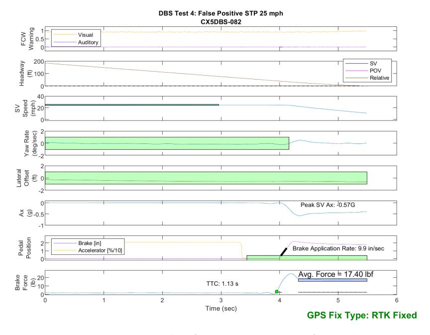
Figure E55. Time History for DBS Run 82, Test 4 - False Positive STP 25 mph
