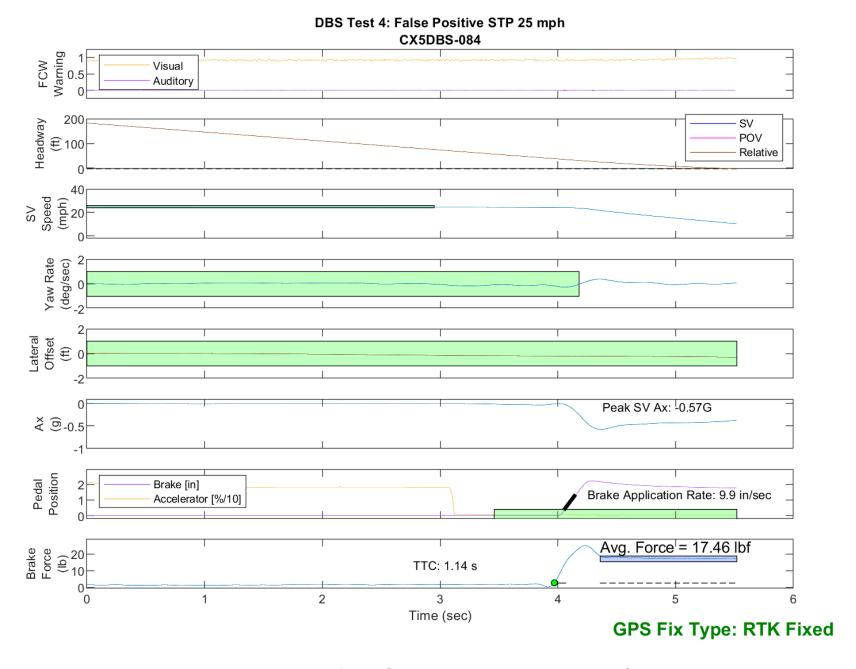
Figure E57. Time History for DBS Run 84, Test 4 - False Positive STP 25 mph
