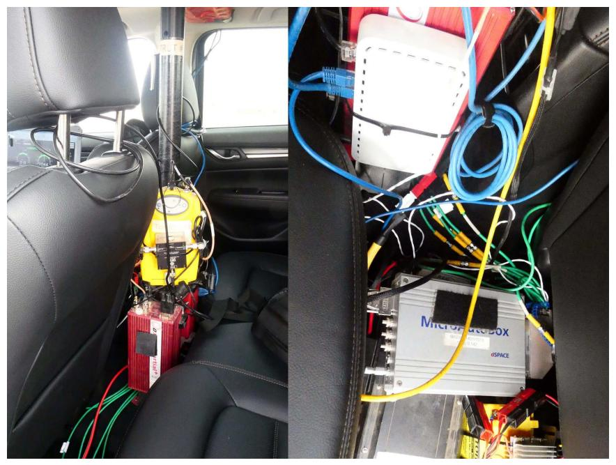
Figure A10. DGPS, Inertial Measurement Unit, and MicroAutoBox Installed in Subject Vehicle A-12
