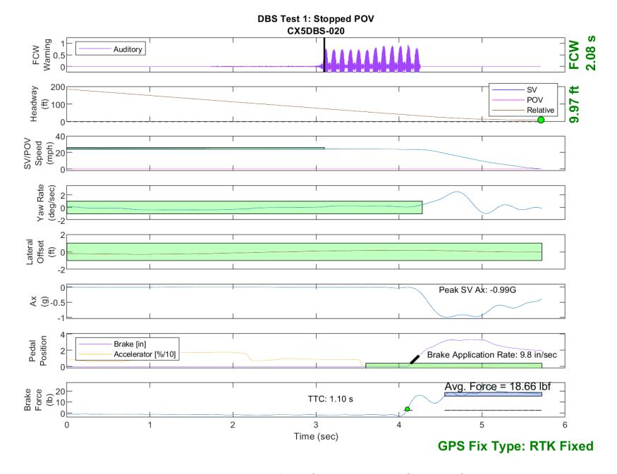
Figure E15. Time History for DBS Run 20, Test 1 - Stopped POV
