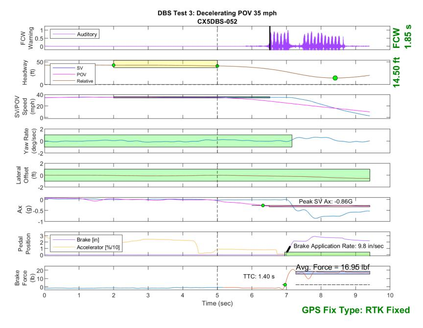
Figure E39. Time History for DBS Run 52, Test 3 - Decelerating POV 35 mph
