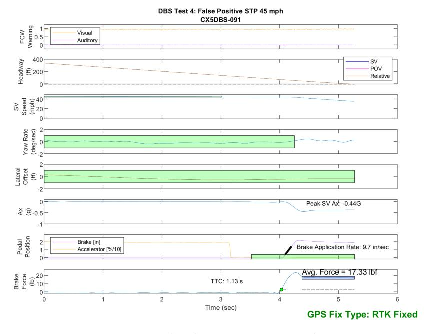
Figure E62. Time History for DBS Run 91, Test 4 - False Positive STP 45 mph
