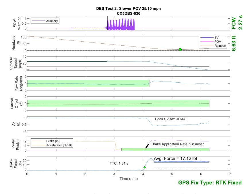
Figure E22. Time History for DBS Run 30, Test 2 - Slower Moving POV 25/10 mph
