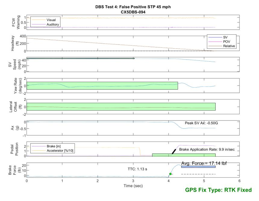
Figure E65. Time History for DBS Run 94, Test 4 - False Positive STP 45 mph
