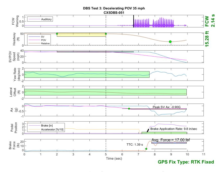
Figure E38. Time History for DBS Run 51, Test 3 - Decelerating POV 35 mph
