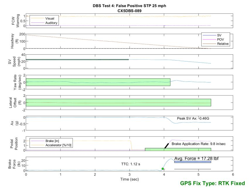
Figure E61. Time History for DBS Run 89, Test 4 - False Positive STP 25 mph
