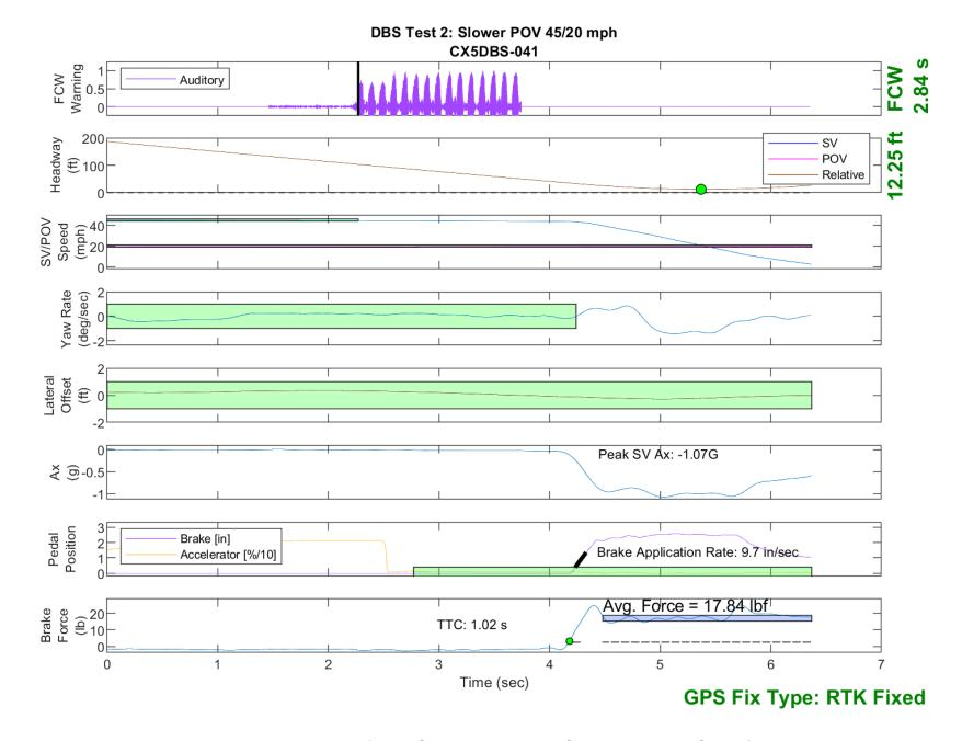
Figure E31. Time History for DBS Run 41, Test 2 - Slower Moving POV 45/20 mph
