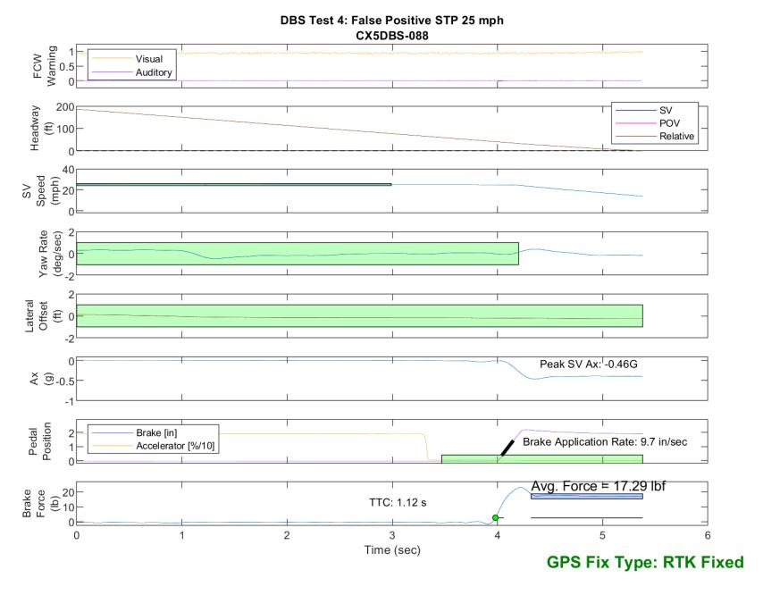
Figure E60. Time History for DBS Run 88, Test 4 - False Positive STP 25 mph
