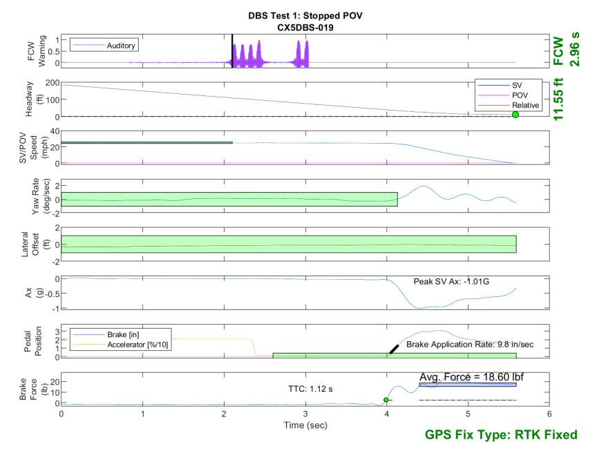
Figure E14. Time History for DBS Run 19, Test 1 - Stopped POV
