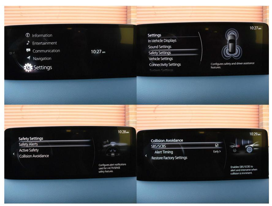
Figure A16. AEB System Setup Menus
