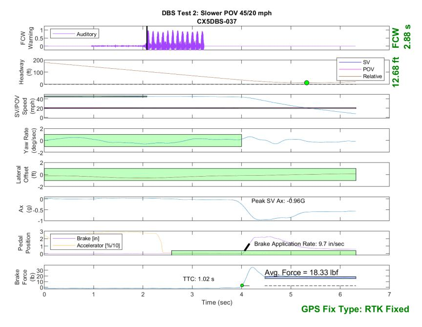
Figure E27. Time History for DBS Run 37, Test 2 - Slower Moving POV 45/20 mph
