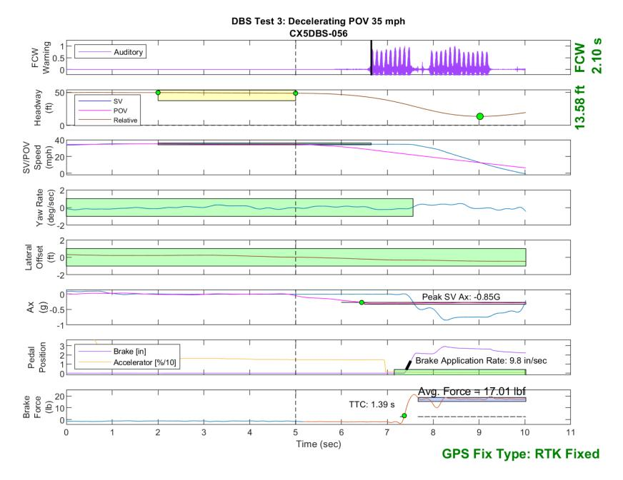
Figure E40. Time History for DBS Run 56, Test 3 - Decelerating POV 35 mph
