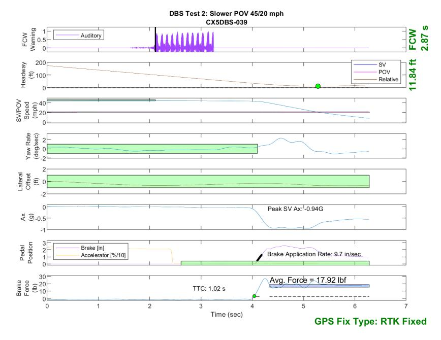
Figure E29. Time History for DBS Run 39, Test 2 - Slower Moving POV 45/20 mph
