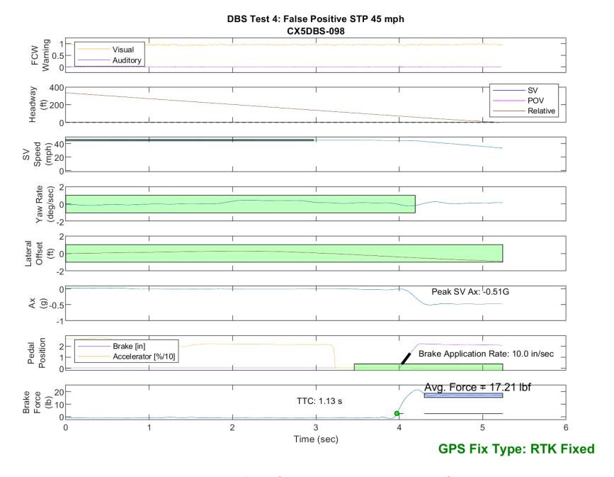
Figure E68. Time History for DBS Run 98, Test 4 - False Positive STP 45 mph
