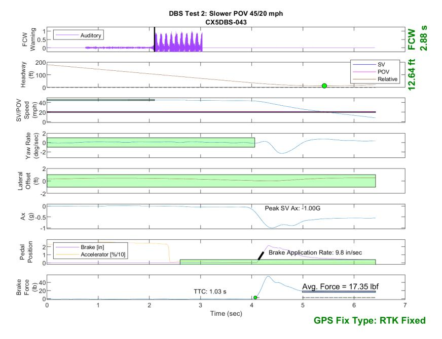
Figure E33. Time History for DBS Run 43, Test 2 - Slower Moving POV 45/20 mph
