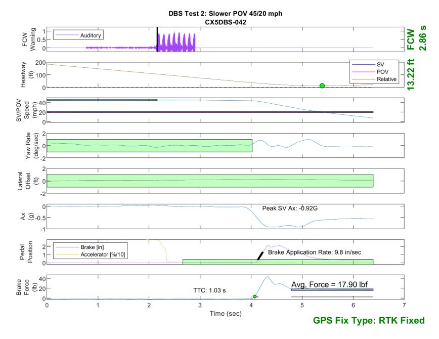
Figure E32. Time History for DBS Run 42, Test 2 - Slower Moving POV 45/20 mph
