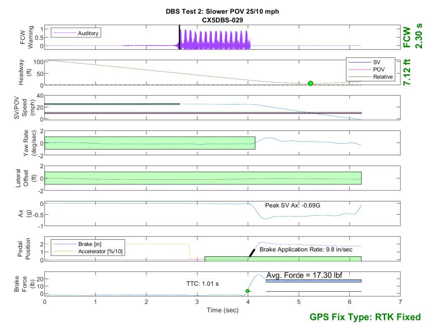
Figure E21. Time History for DBS Run 29, Test 2 - Slower Moving POV 25/10 mph
