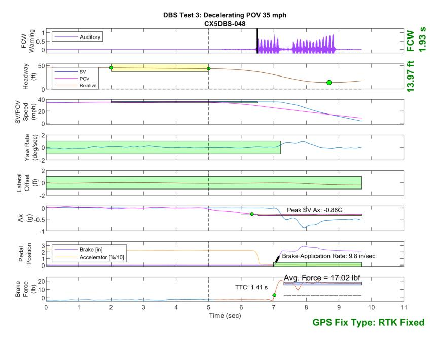
Figure E35. Time History for DBS Run 48, Test 3 - Decelerating POV 35 mph
