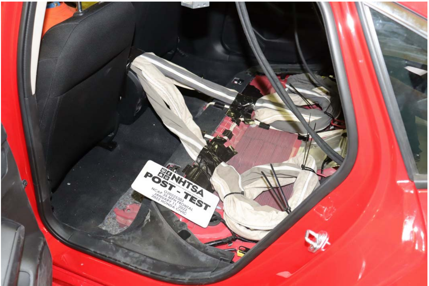
Photo No. 029 - Post-Test Dummy Cable Routing
