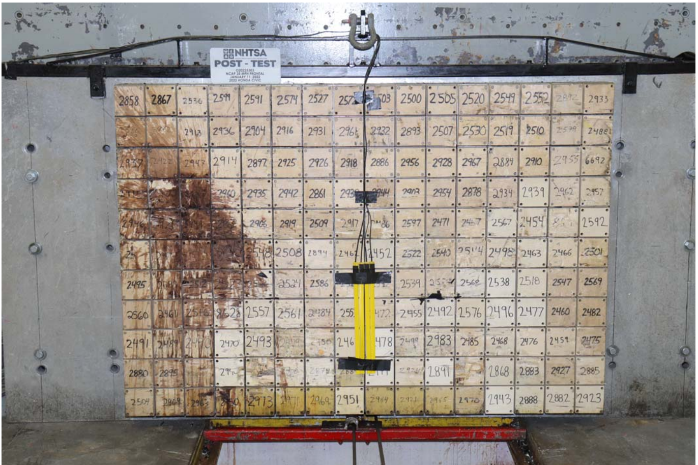
Photo No. 003 - Post-Test Load Cell Wall
