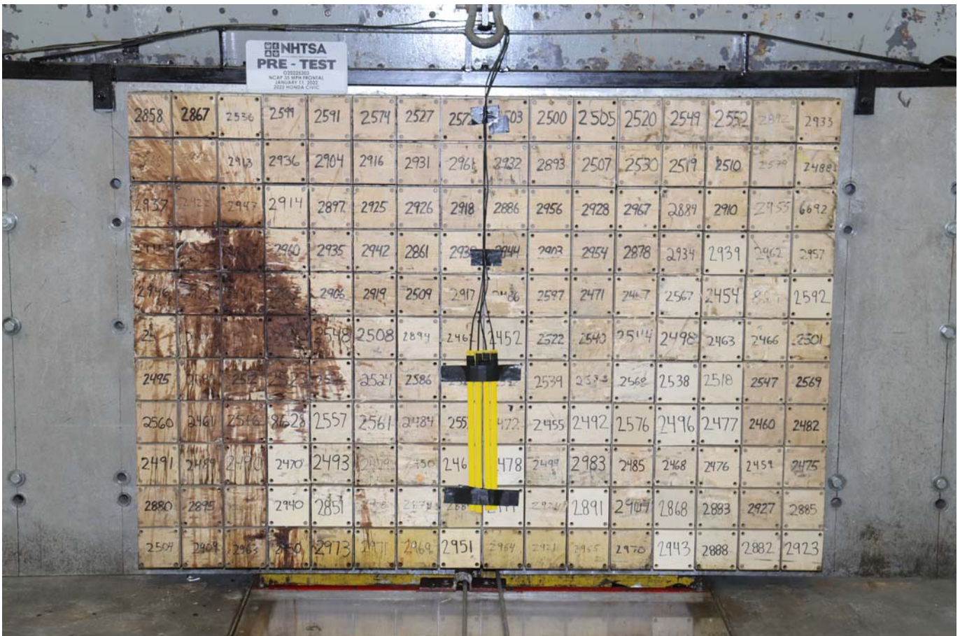
Photo No. 002 - Pre-Test Load Cell Wall
