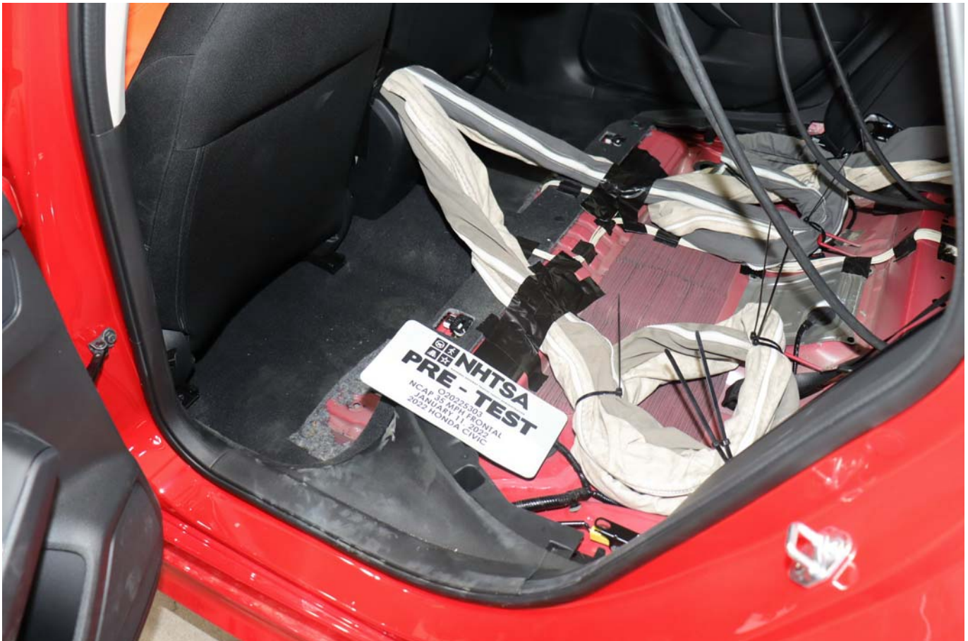
Photo No. 028 - Pre-Test Dummy Cable Routing
