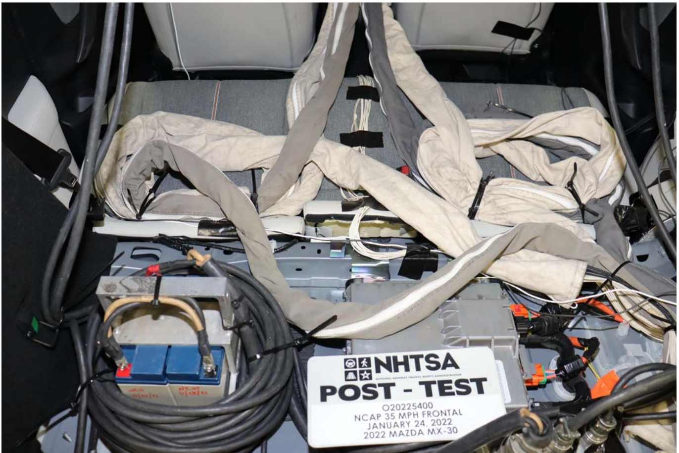
Photo No. 029 - Post-Test Dummy Cable Routing
