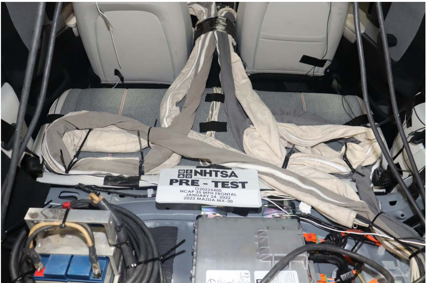
Photo No. 028 - Pre-Test Dummy Cable Routing
