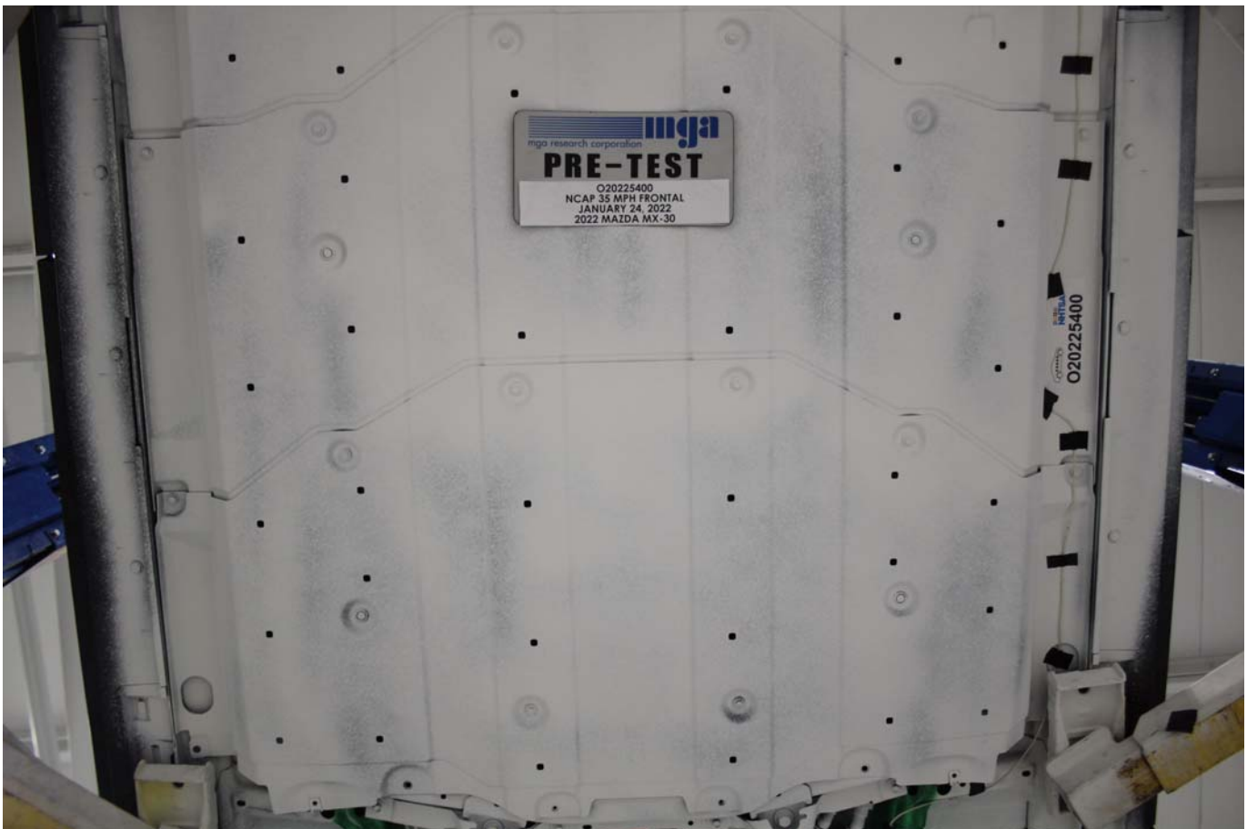
Photo No. 305-09 - Pre-Impact View of Propulsion Battery
