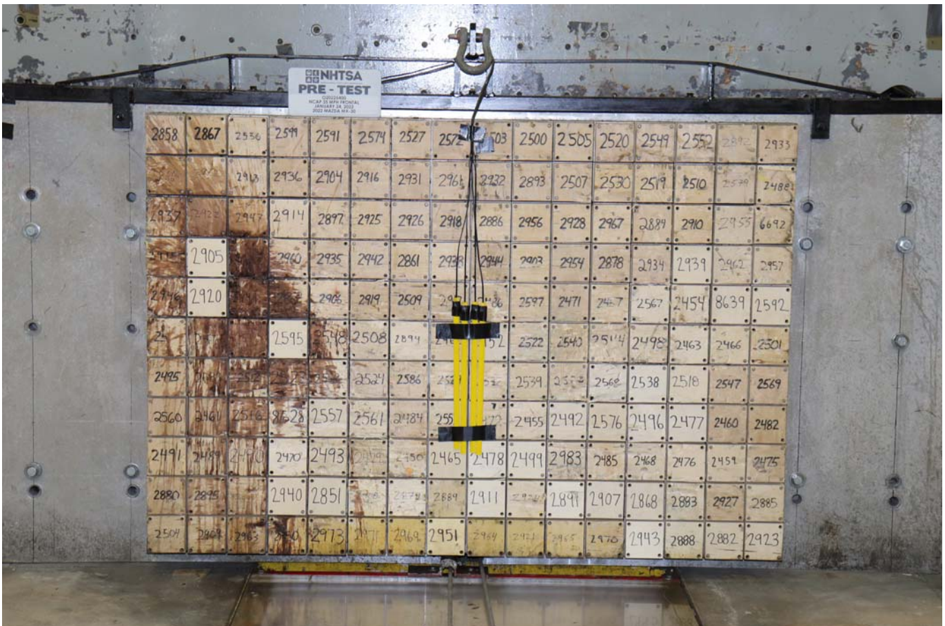
Photo No. 002 - Pre-Test Load Cell Wall
