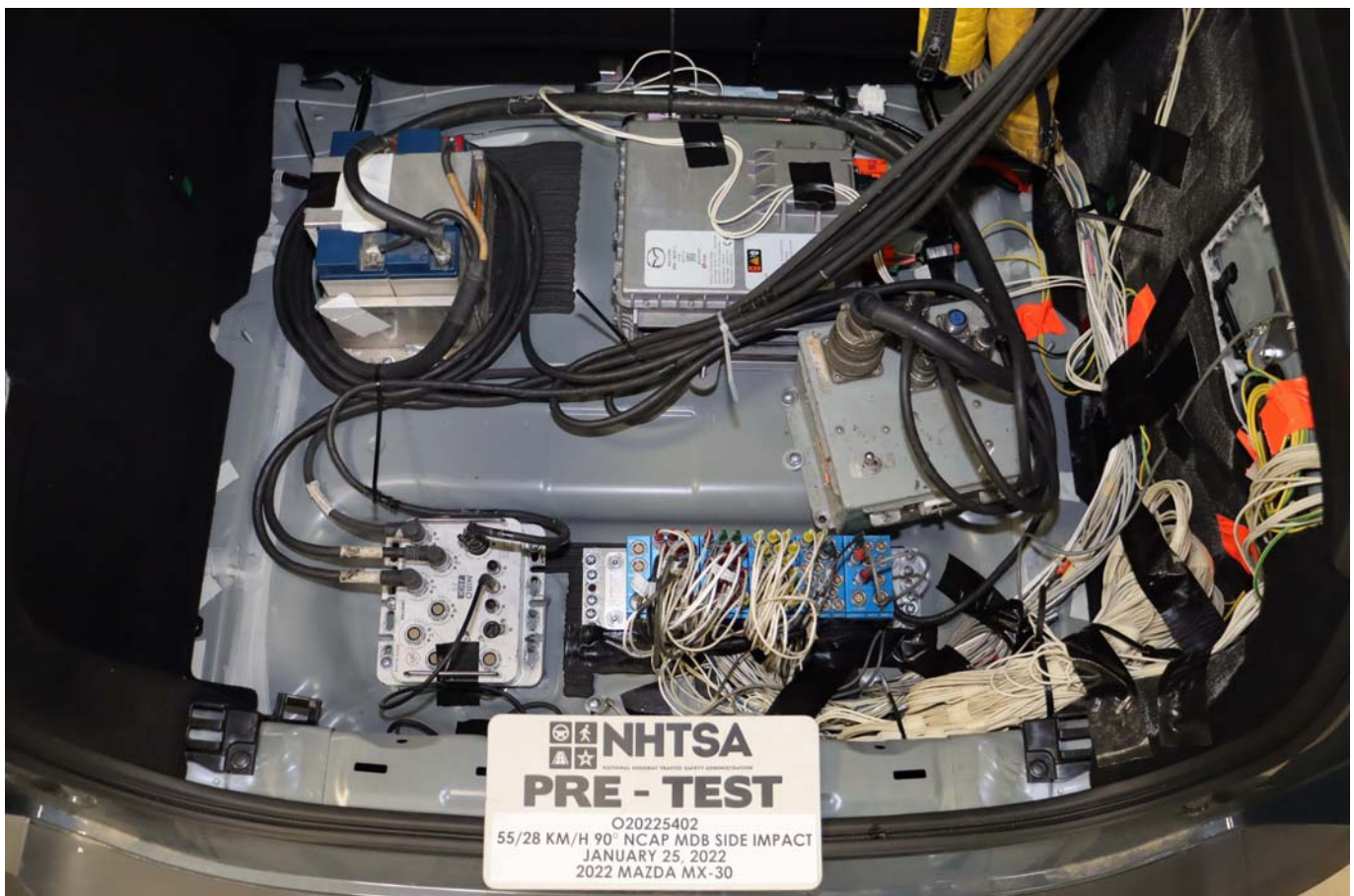
Photo No. 094 - Pre-Test Ballast View
