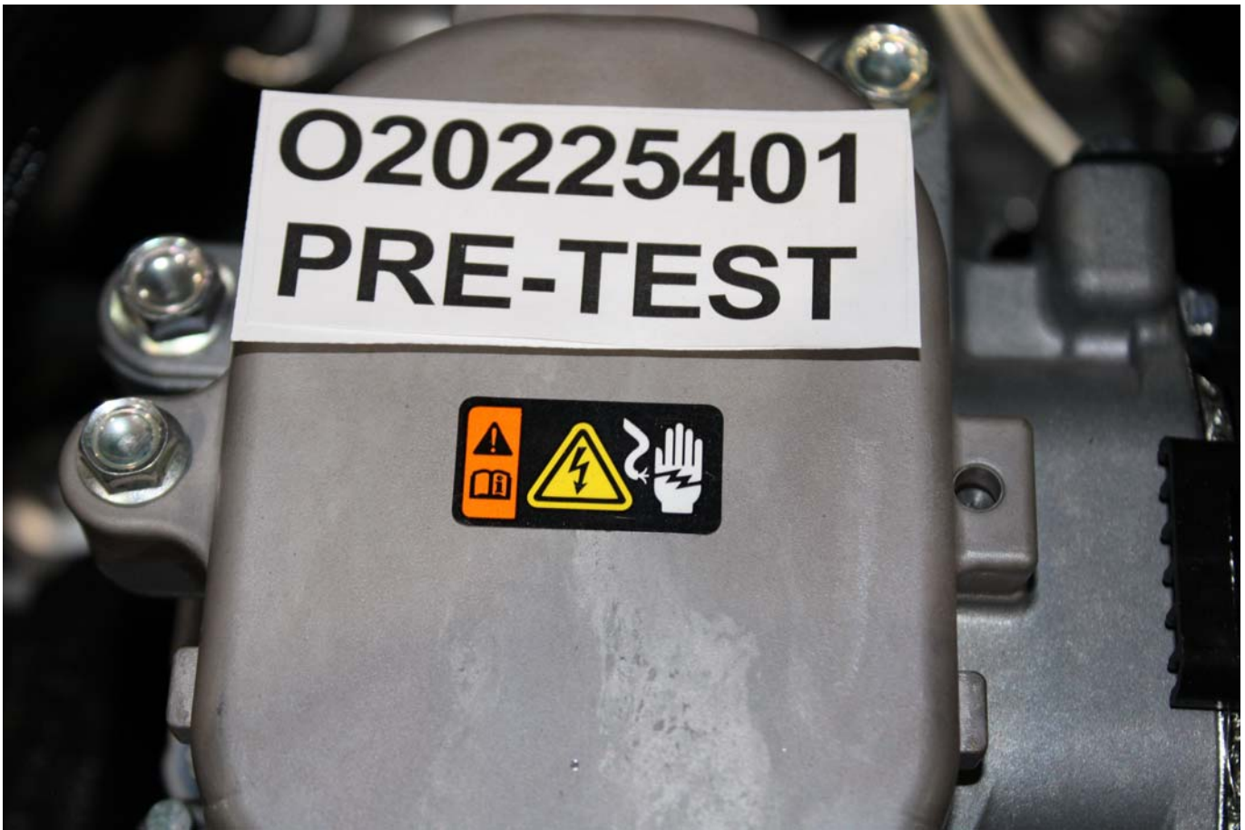
Photo No. 305-02 - Power Inverter Warning Label
