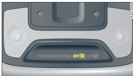
Fig. 1 Headliner: indicator light to display the status of the front passenger's airbag
