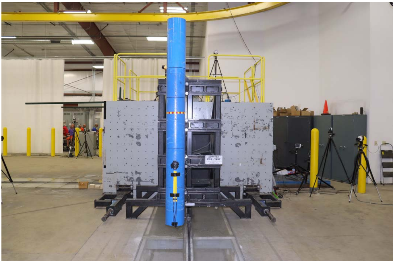
Photo No. 059 - Pre-Test Pole Barrier Front View
