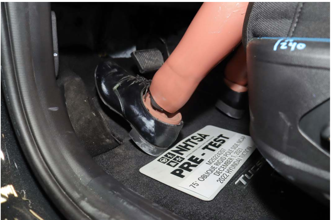
Photo No. 032 - Pre-Test Placement of Dummy Feet
