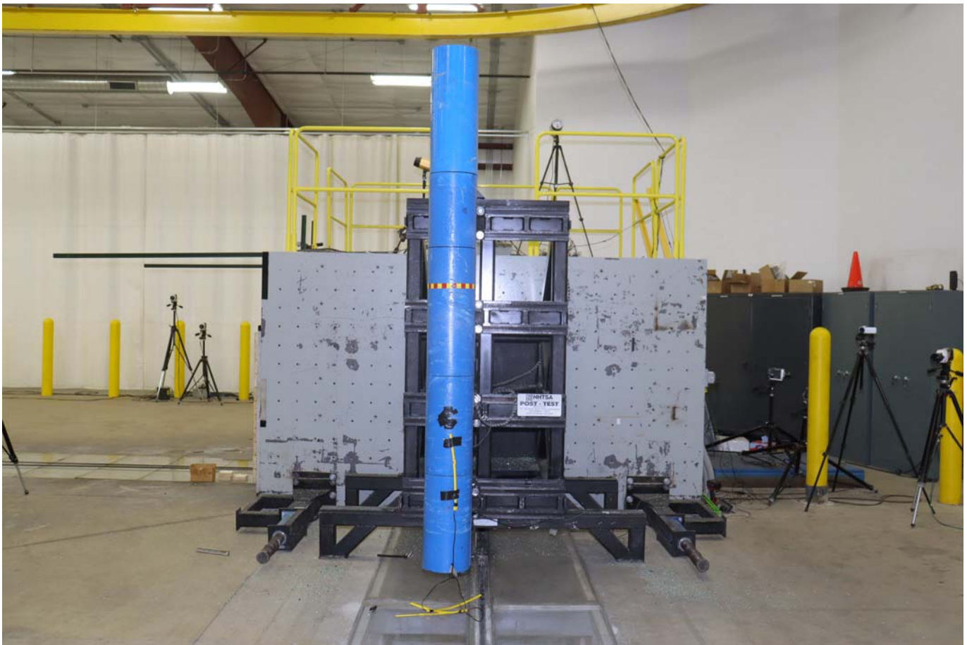
Photo No. 060 - Post-Test Pole Barrier Front View
