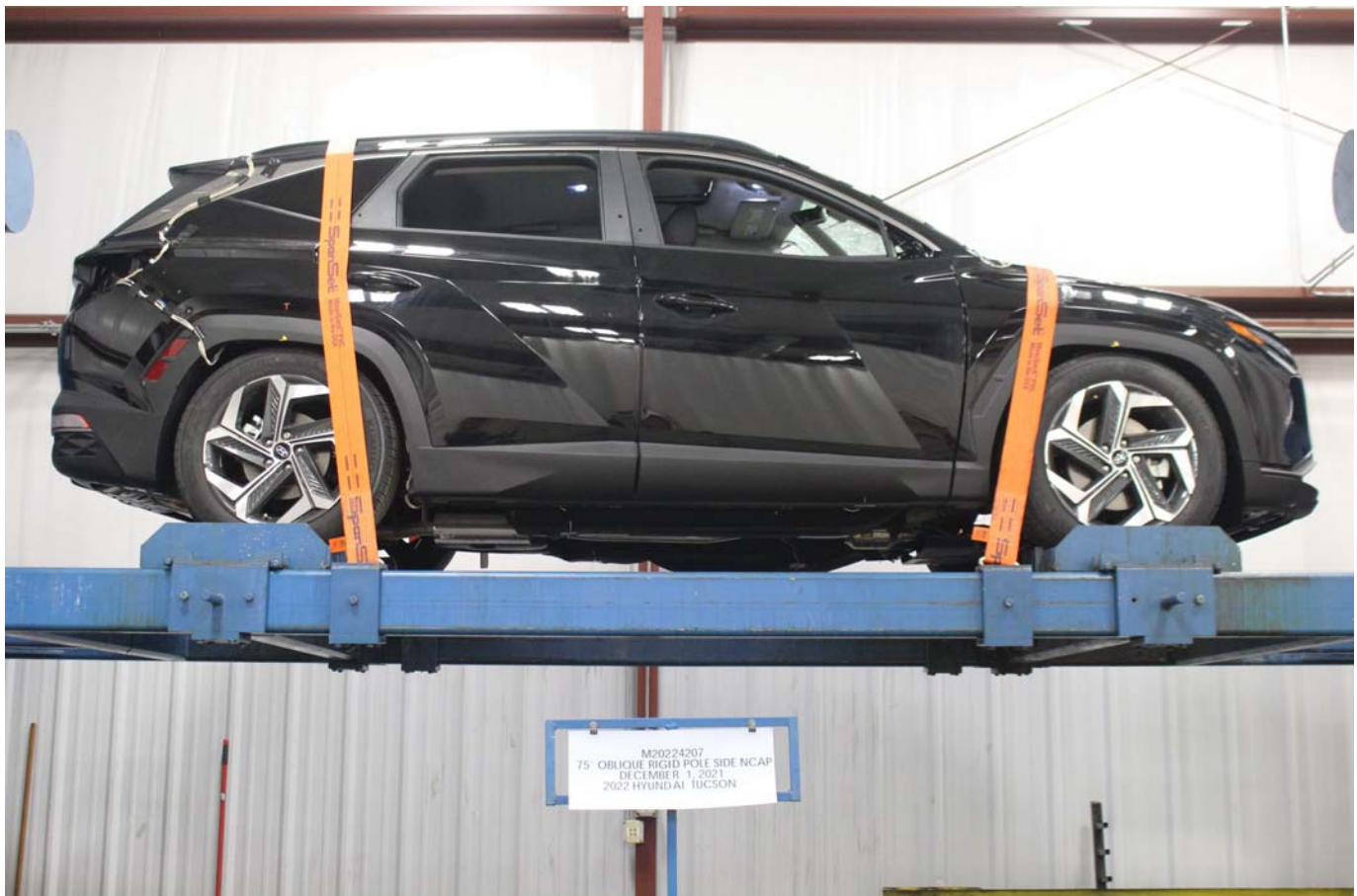
Photo No. 065 - FMVSS Photo No. 301 Static Rollover 0 Degrees
