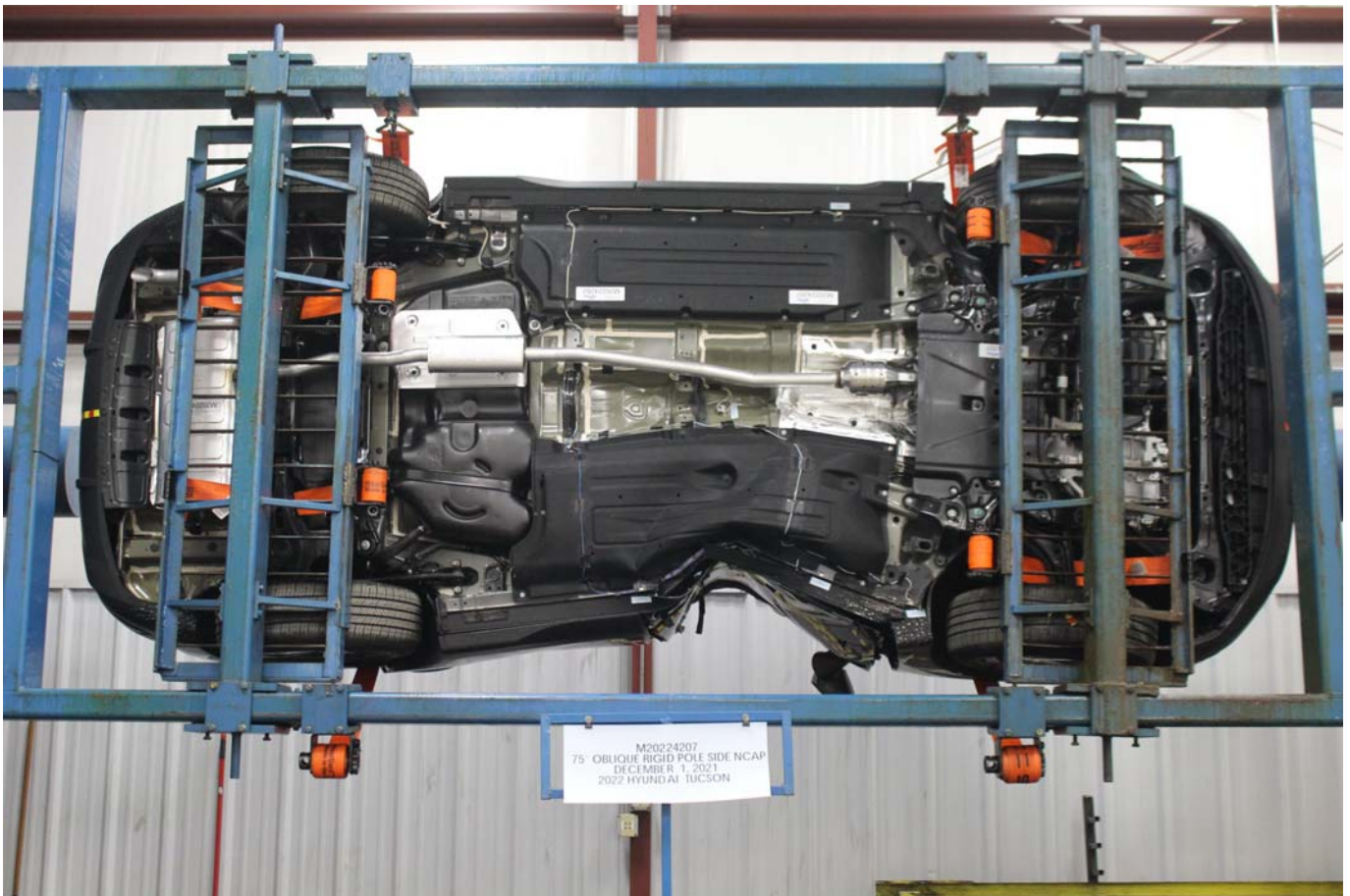
Photo No. 066 - FMVSS Photo No. 301 Static Rollover 90 Degrees
