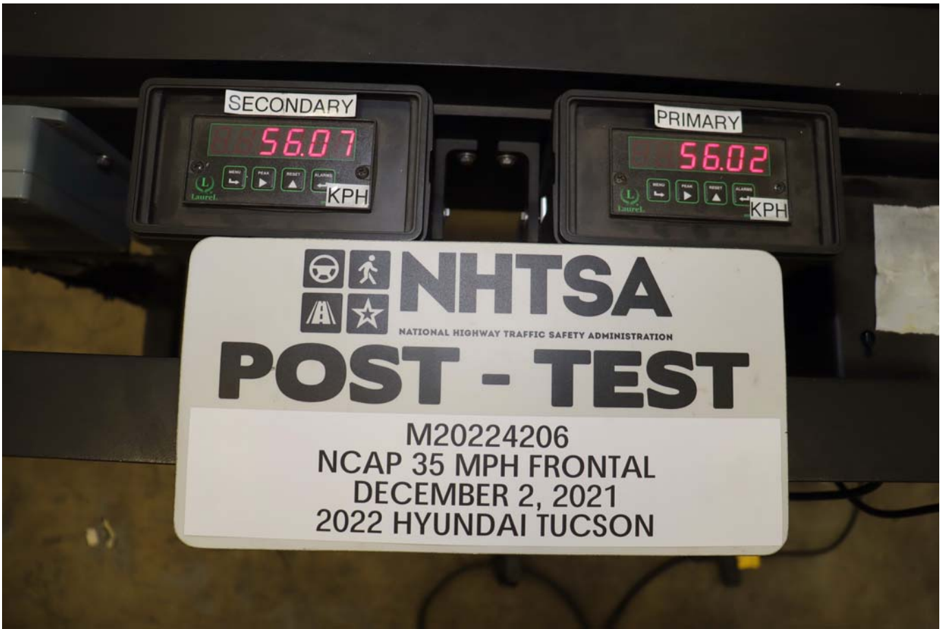
Photo No. 076 - Post-Test Speed Trap Read-Out
