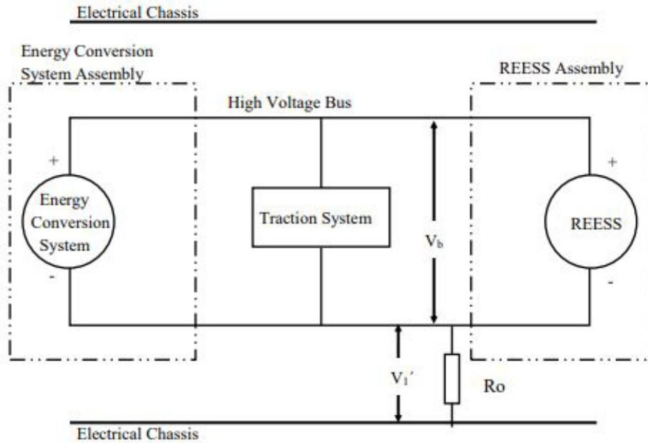
5. Calculate the electrical isolation ( $R_i$ ) according to the following formula:
