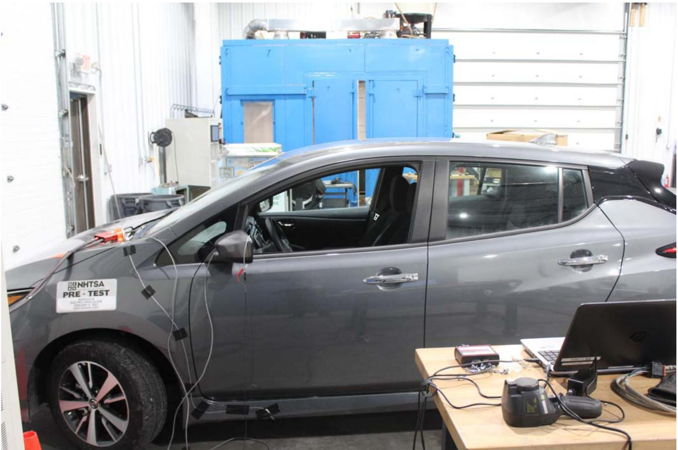
Photo No. 018 - Overcharge Test Setup
