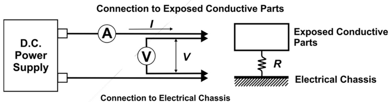
3. Measure the current "I" and voltage "V" between the test location and the electrical chassis. Calculate the resistance between the test location and the electrical chassis using the following formula:  $R = V / I$
