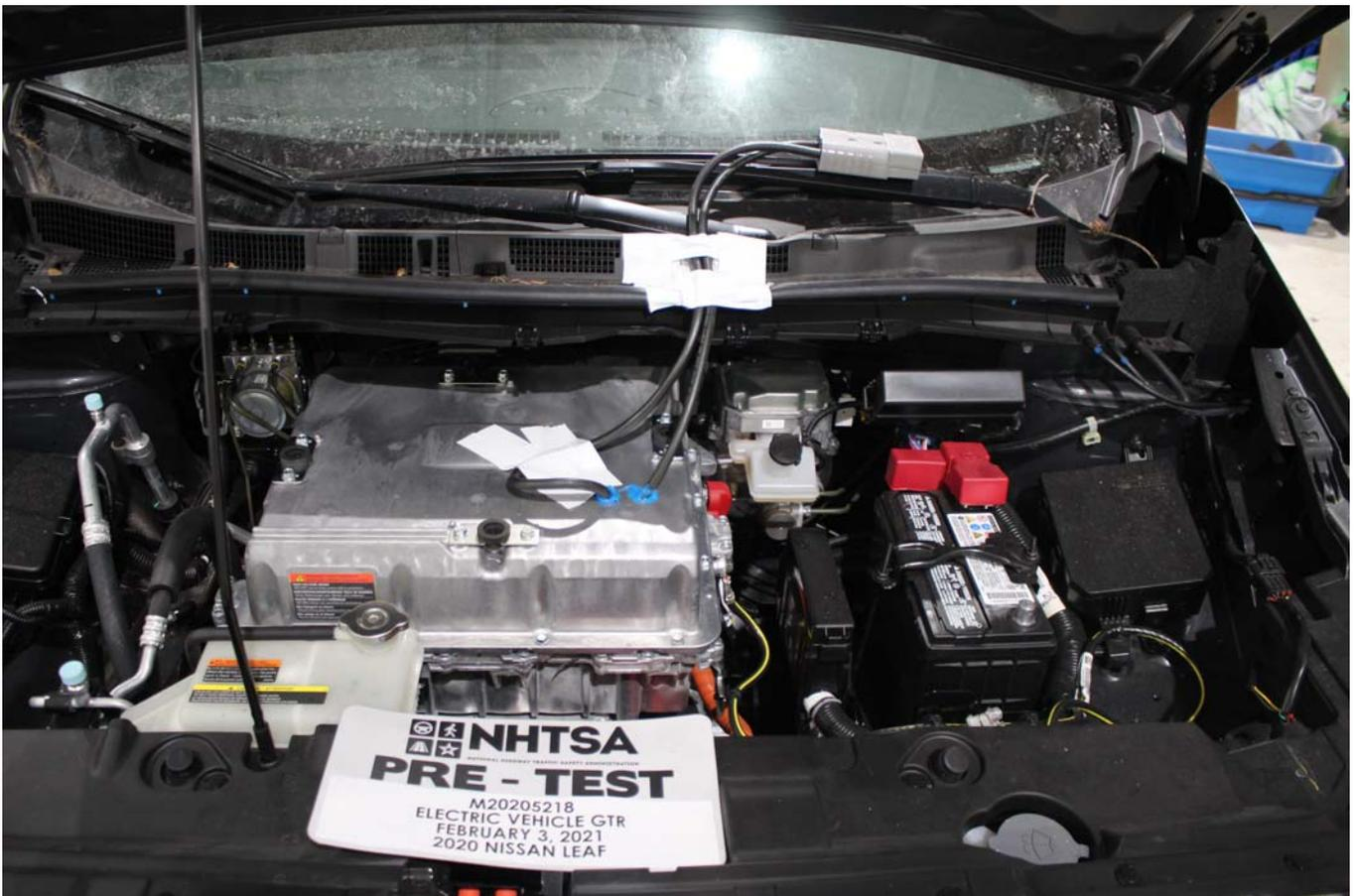
Photo No. 014 - External Short Circuit Breakout Harness
