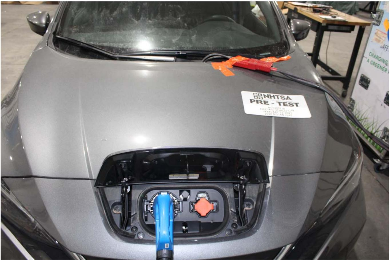
Photo No. 027 - Overcurrent Test Setup
