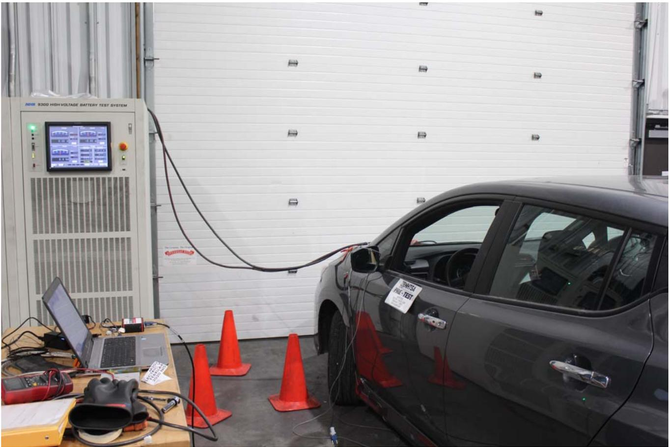
Photo No. 021 - Over-discharge Test Setup
