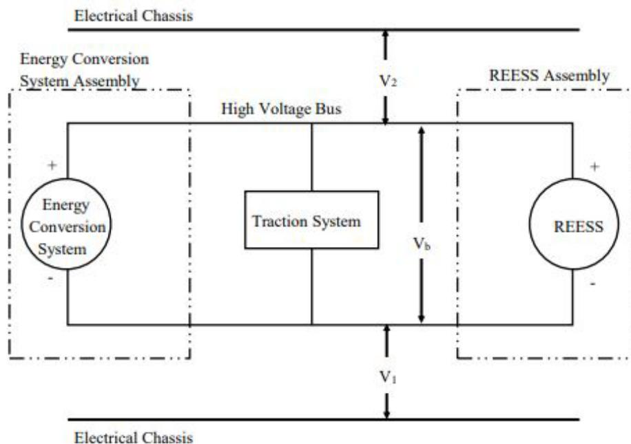
3. Measure and record the voltage ( $V_1$ ) between the negative side of the high voltage bus and the electrical chassis and voltage ( $V_2$ ) between the positive side of the high voltage bus and the electrical chassis (see Figure 2).
