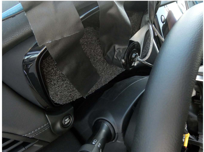
Figure A10. Sensors for Detecting Auditory and Visual Alerts
